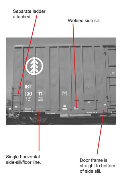
Figure 3: End Identification of Gunderson 6269 Box Cars
