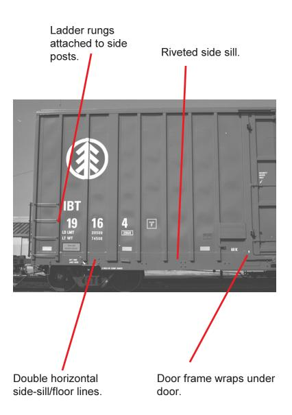
Figure 2: Side Identification of Trenton Works 6269 Box Cars
