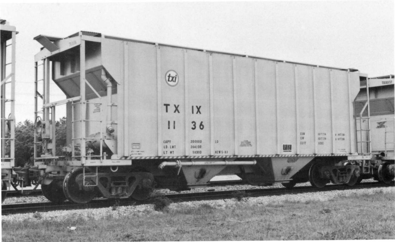
**Portec 3200 cf FG design** (above). TXIX 1136 was built in April 1982 as part of the TXIX 1101-1142 series by Portec's GRO WGA (Winder GA). The car uses a fluidized-gravity system for unloading. TXIX is a reporting mark for Texas Industries.
