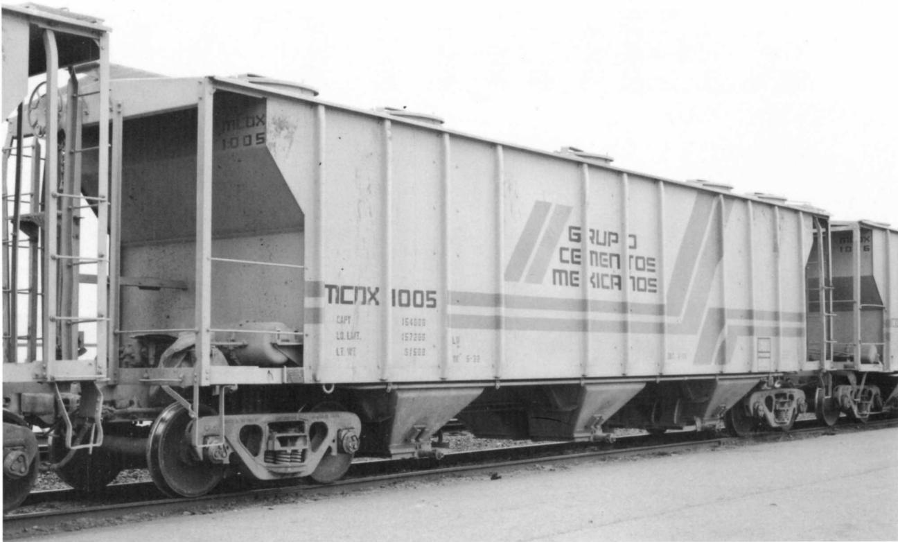
**MCDX 1005** (above) is part of a series of fifty 70-ton three-bay covered hoppers being operated by Grupo Cementos Mexicanos (MCDX is a reporting mark of Sunbelt Cement). Number series, MCDX 1000-1049. Built in 1958. This car has a stencilled cubic-foot capacity of 2,927. Outside length, 49'11".
