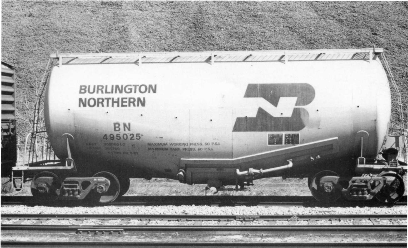
**GATX 207A60W design** (above). BN 495025 is essentially the same type of car as the Baroid car. This one is rated at 2,800 cubic-foot, too. Series, BN 495000-495049 (CB&Q 84950-84999). Outside length, 41'3".
