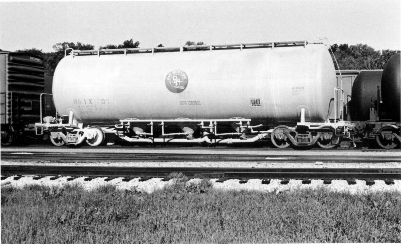
**Union Tank 207A40W design** (above). The one and only RMIX 200. Built in April 1971. Cubic-foot capacity on this is 3,000. RMIX is a reporting mark for Ready Mixed Concrete Co.
