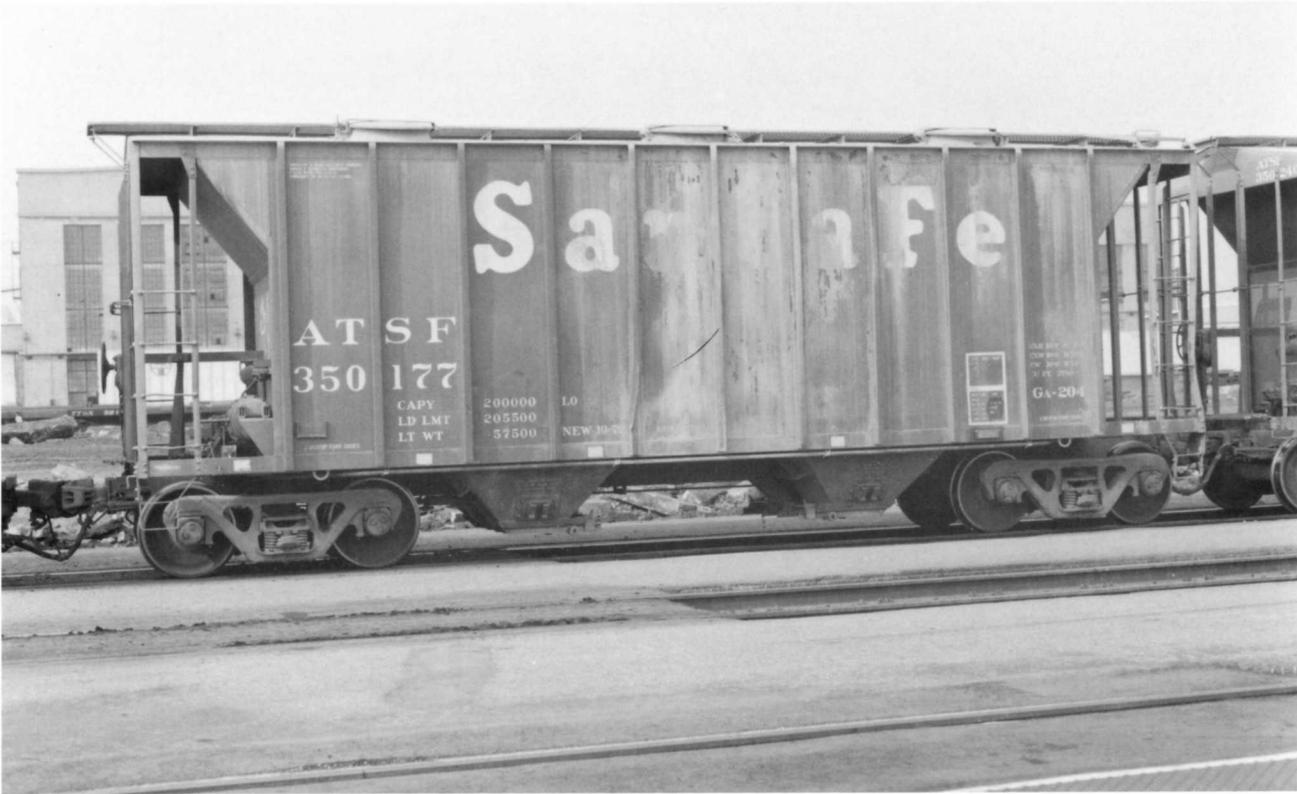
**Greenville 2700 cf design** (above). ATSF 350177 is pretty much the same design as the ANAX/NAHX 2917 cf car on the previous page. Both cars have almost the same features. Note that on this car the top end of the hopper falls just inside the ladder. On the ANAX car the top hopper ends go past the inner ladder stile. Outside length is 41'11".
