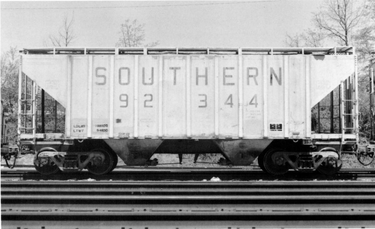
**PS 3000 cf design** (above). Southern 92344 was built in January 1981 as part of the series 92100-92399 (300 cars). Outside length, 41'11". The standard PS 3000 design has eleven side stakes, clerestory roof, and a straight side sill.
