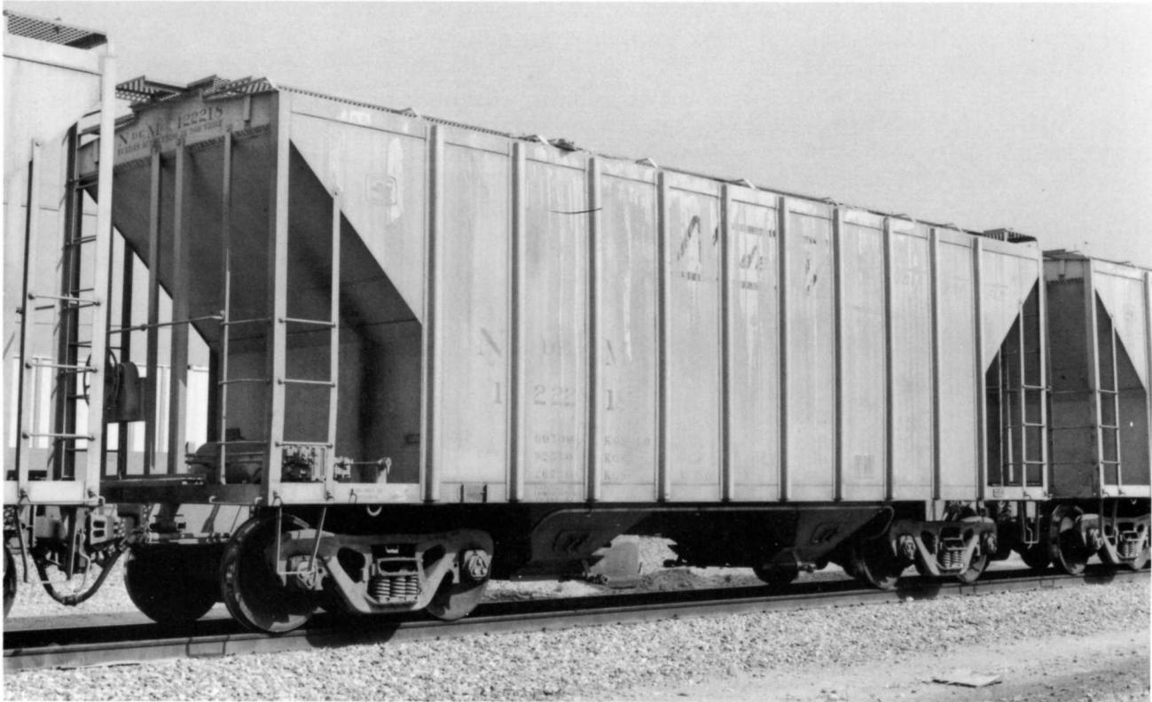
**CNCF 3000 cf design** (above). NdeM 122218 was built in 1986 as part of the NdeM 122000-122299 series. Though it looks a little like the PS design with the clerestory roof there are a number of differences including only ten ribs and a much different end platform arrangement.
