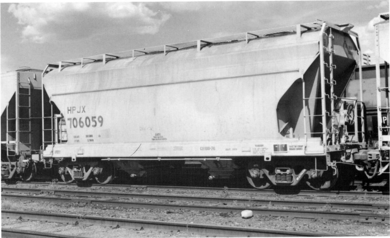
ACF 2970 cf design (above). HPJX 706059 is a former Missouri Pacific car. Originally from the TP 706000-706099 series. Built in March 1967 at Milton. Outside length, 39'8". Equipped with four 30" hatches and gravity outlets. HPJX is a reporting mark of HELM-Pacific Leasing.
