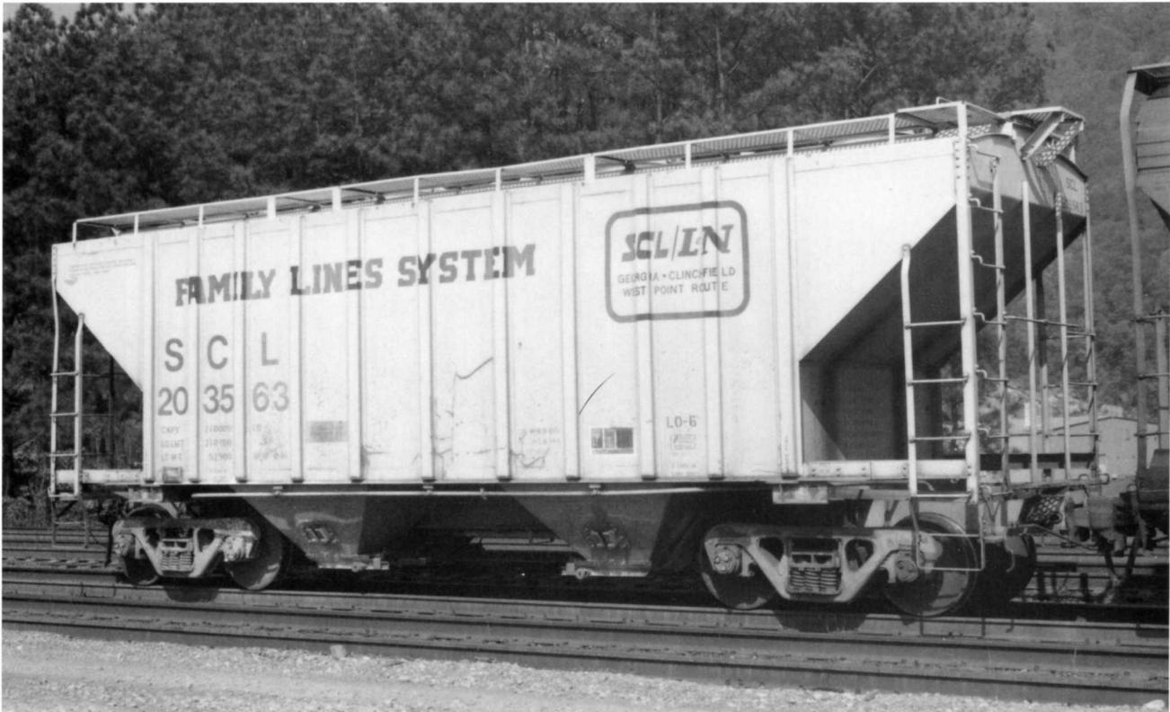
**PS 3000 cf design** (above). SCL 203563 is part of the SCL 203500-series built for cement and phosphate service. This car was built in August 1981 at Bessemer AL.
