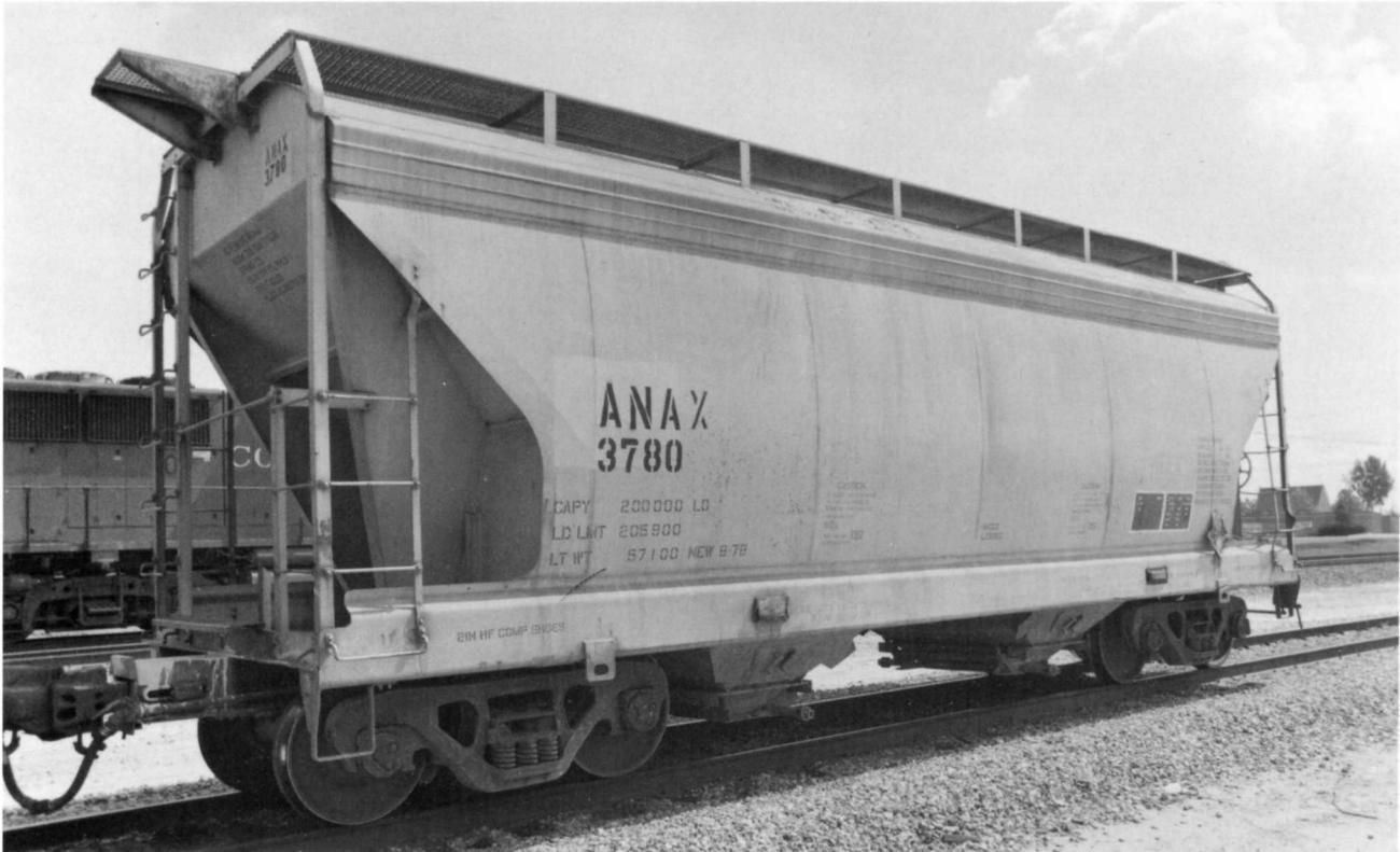
**ACF 2980 cf design** (above). ANAX 3780 was originally built as part of the IMCX 6500-6539 series in August 1978. Shown here as part of the series, ANAX 3700-3882 which includes several other designs of nearly the same size. ANAX is a reporting mark for EXCEL Railcar Corporation (Naperville IL).
