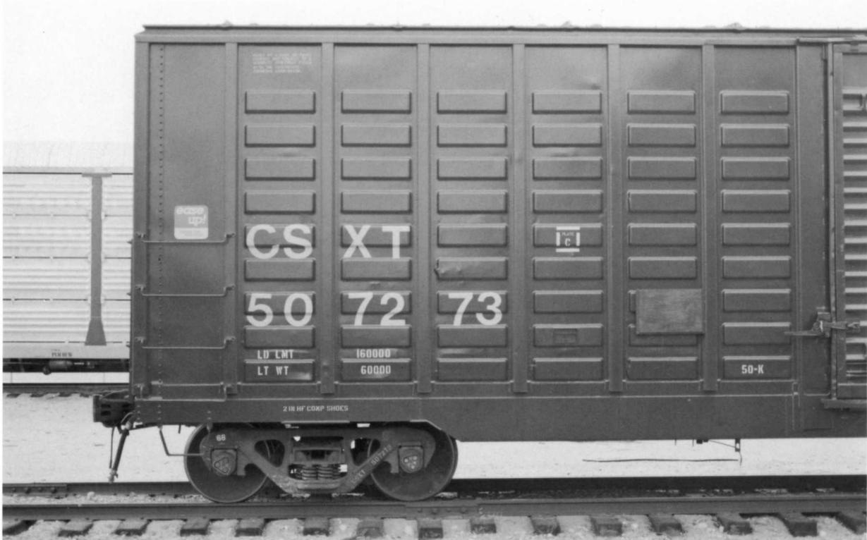
**CSXT 507273** (Above). Left side detail. This is only a 70-ton car - note the 220,000 GRL (160,000 lb load limit + 60,000 lbs light weight).
