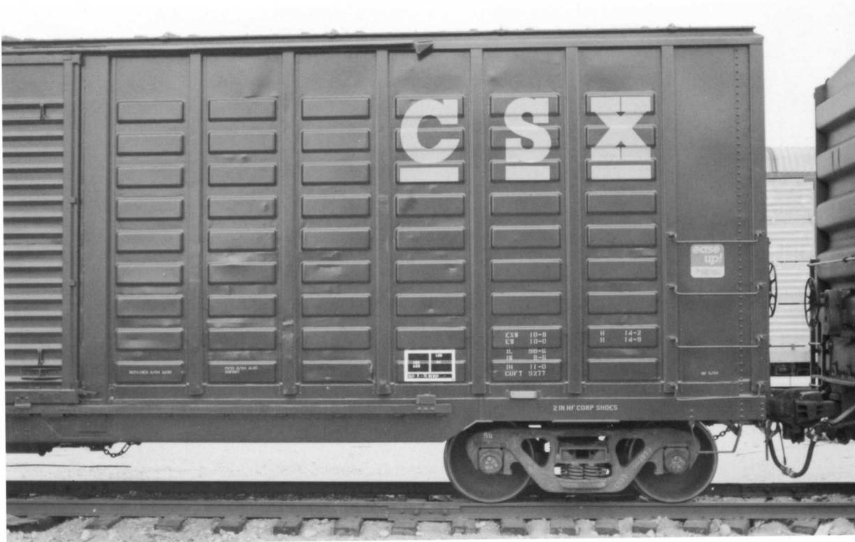
**CSXT 507273** (Above). Right side detail. Note the stencilled capacity is 5,277 cubic-foot. The car was repaired at the Nashville shop in June 1994, then sent to ALRC for painting in August 1994.
