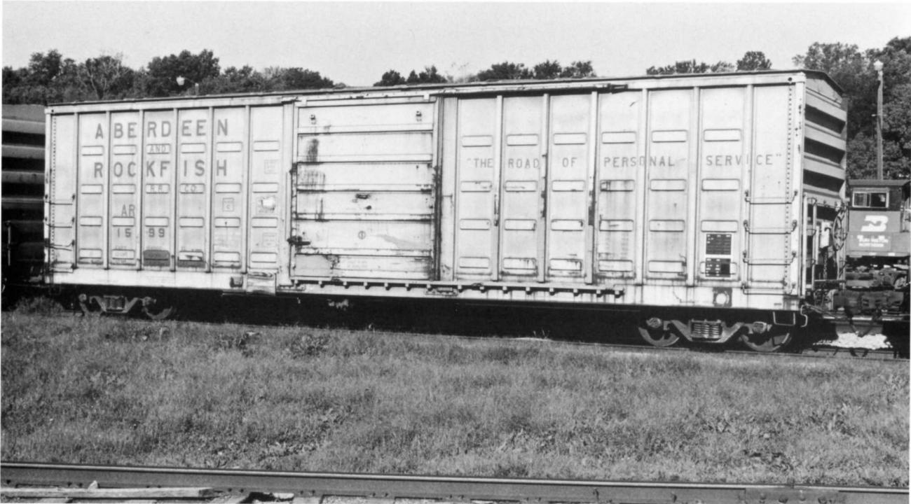
**AR 1599** (Above) is the last car of the series AR 1500-1599 (100 cars). It was built by SIECO's Ashland City plant in 1979. Note the four widely spaced rows of waffles. The ends are non-terminating (recessed) riveted to the sides (instead of welded). *Mike Foley* photo.
