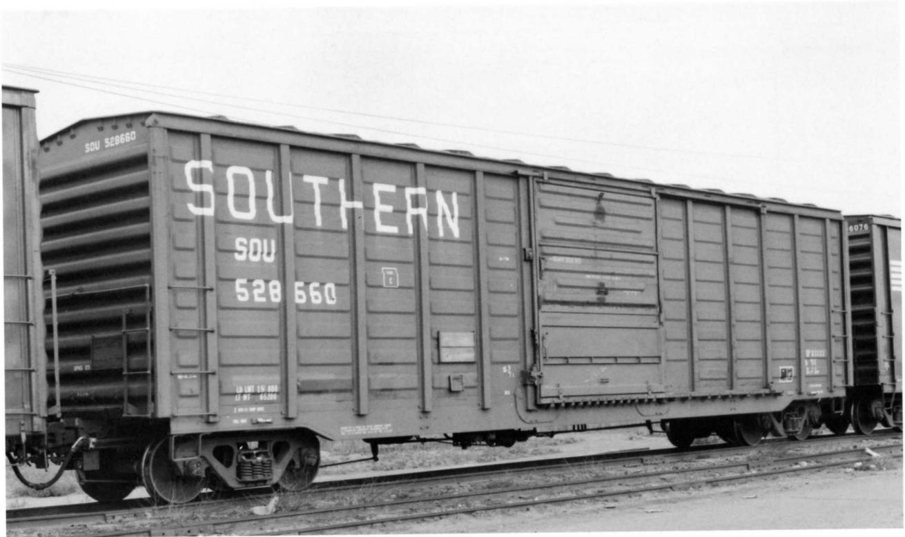
**SOU 528660** (Above) was built by Pullman-Standard a part of the SOU 528300-529099 (800 cars). The car is a 50'6" IL Plate C box car. Note the door has been rebuilt with a new bottom replacing the original PS style corrugated door.
