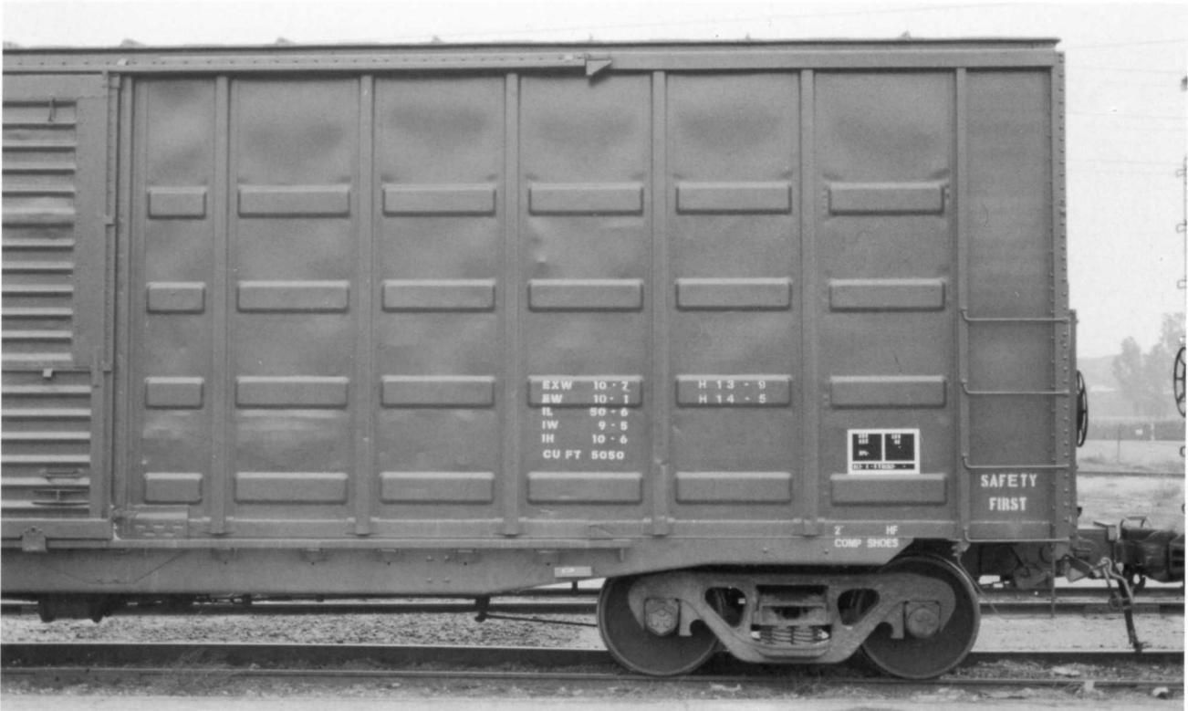
**BPRR 1222** (Above). Right side detail. Each of the cars have a 5,050 cubic-foot capacity. These are 50'6" IL Plate B box cars.
