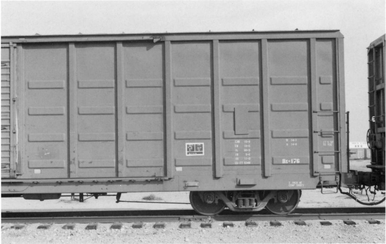
**ATSF 611409.** (Above). Detail of right side. Cubic-foot capacity is stencilled as 6,348. Note the large jack pad on the side sill just above the truck.
