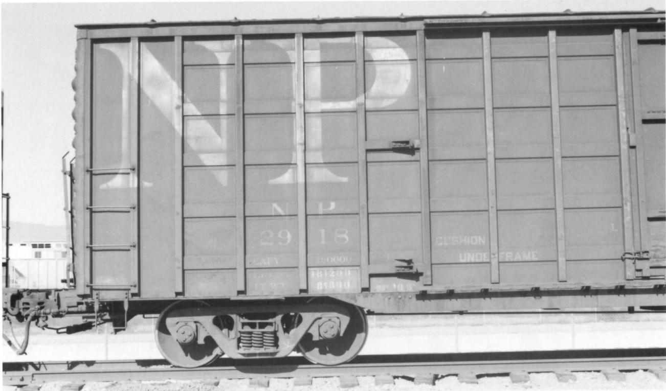
**NP 2918.** (Above). Left side detail showing stenciling indicating a cushioned underframe. Load limit on this car is 181,200 lbs (263,000 GRL / a.k.a "100-ton" car).
