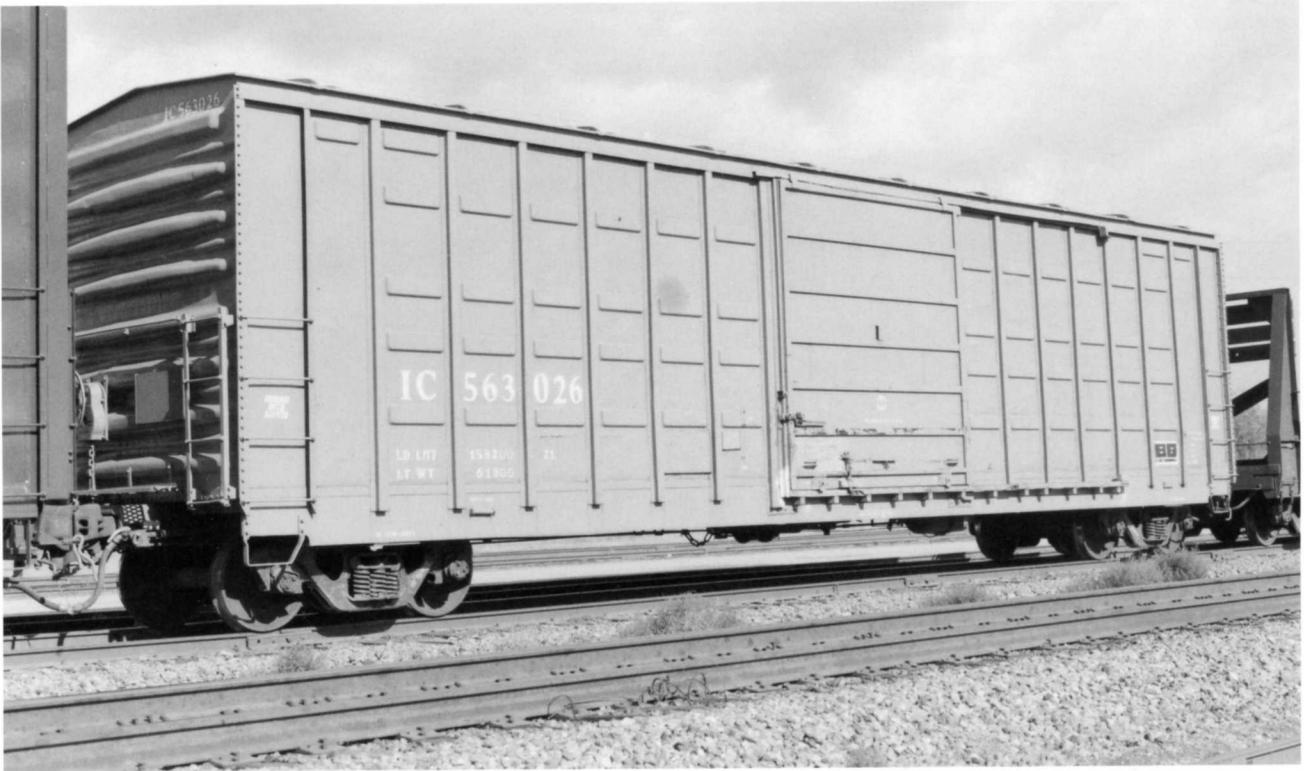
**IC 563026** (Above) was built in September 1969. Again, four rows of waffles plus two in each of the upper corners (but, shifted over one panel). Note the recessed stamped corrugation end.
