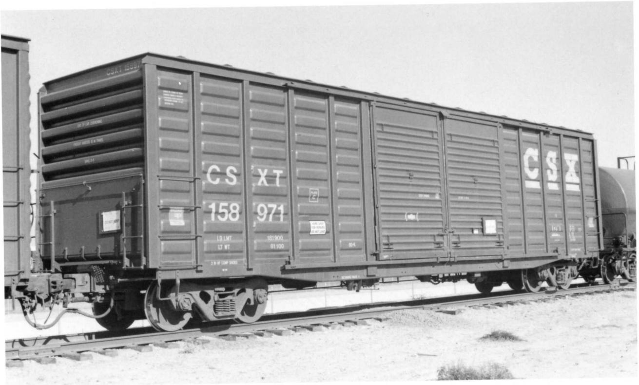
**CSXT 158971.** (Above). This is a 52'6" IL Plate C box car. Door opening is 16'0" x 10'4" (WxH). There are nine rows of waffles dispersed between the ten side posts. Note the flat roof and lower solid end sheet. The car has a heavy-duty 60K floor and loaders for paper loading.
