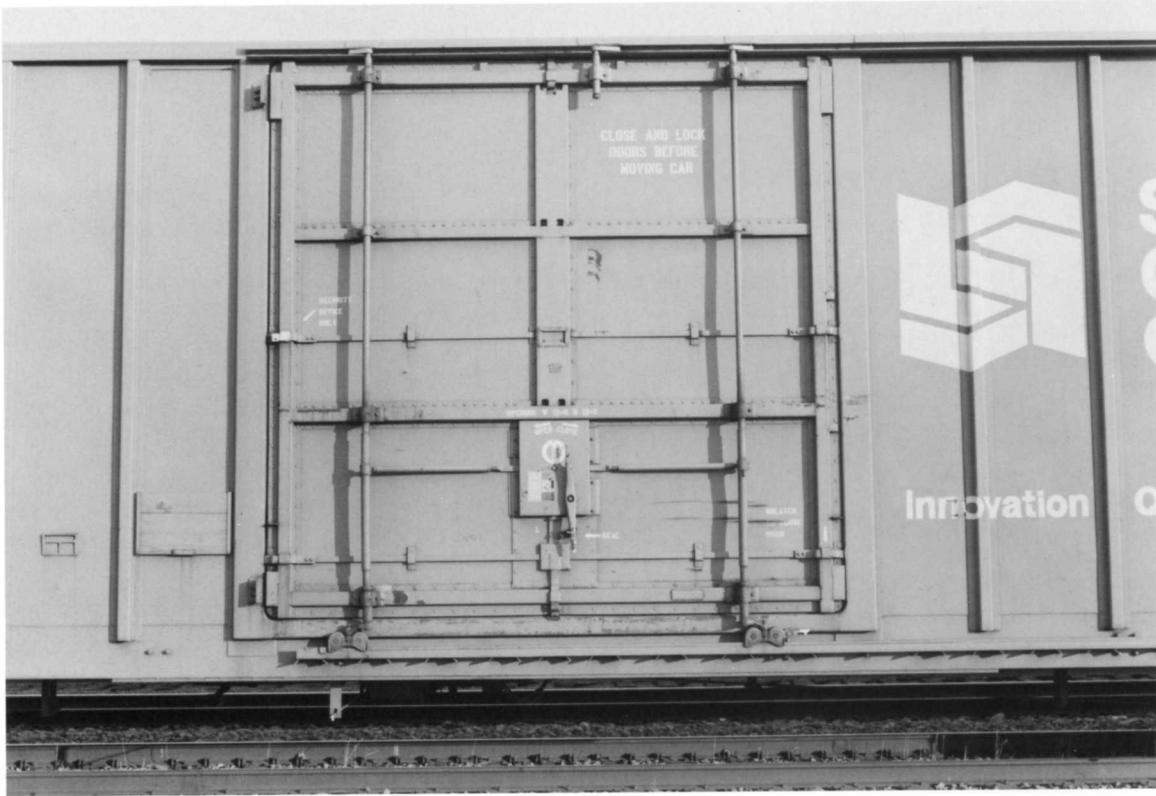
**AG 1018.** (Above). Detail of plug door and door area. This is a Youngstown (YSD) door. Note the frame surrounding the door goes just below the floor line. The bottom of the door itself is at the floor level.
