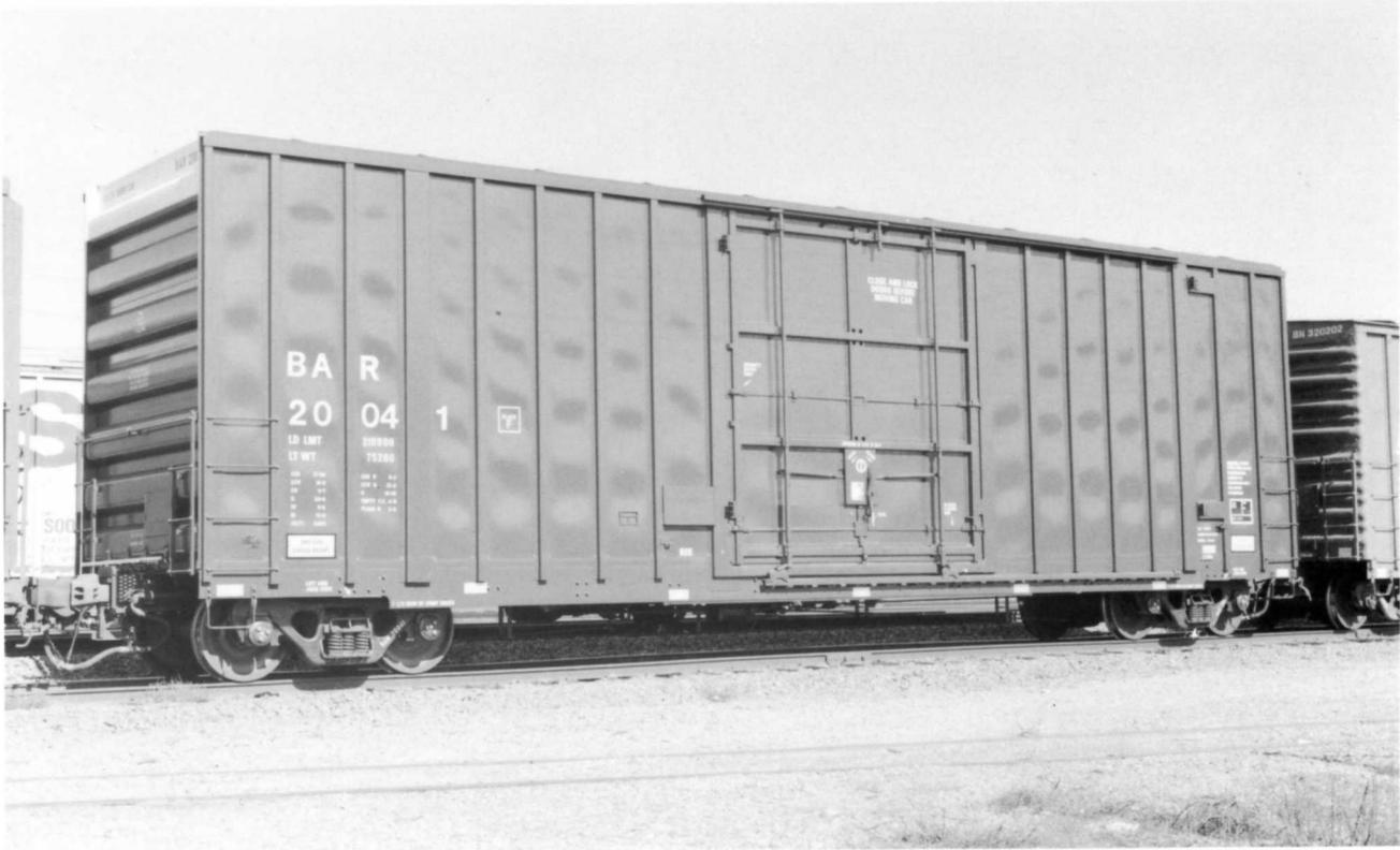
**BAR 20041.** (Above). Gunderson built this car in December 1994. Series, BAR 20000-20078 (79 cars). Livery is brown and white. These are 50'6" Plate F box cars. Door opening, 10'0" x 12'4" (WxH). Note the 2/2/3 end, fourteen side posts, and flat roof. Photographed in Colton, CA.
