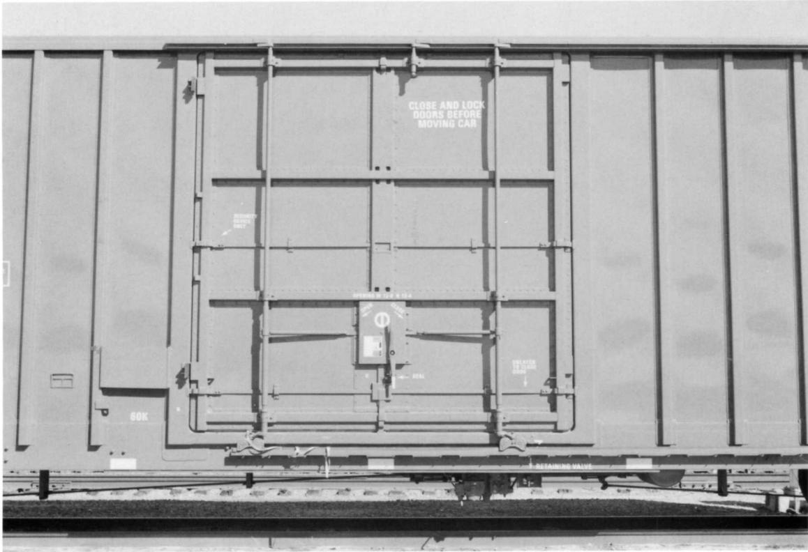
**BN 287227.** (Above). Detail of plug door and door area. This car has a 12'0" x 12'4" (WxH) plug door.
