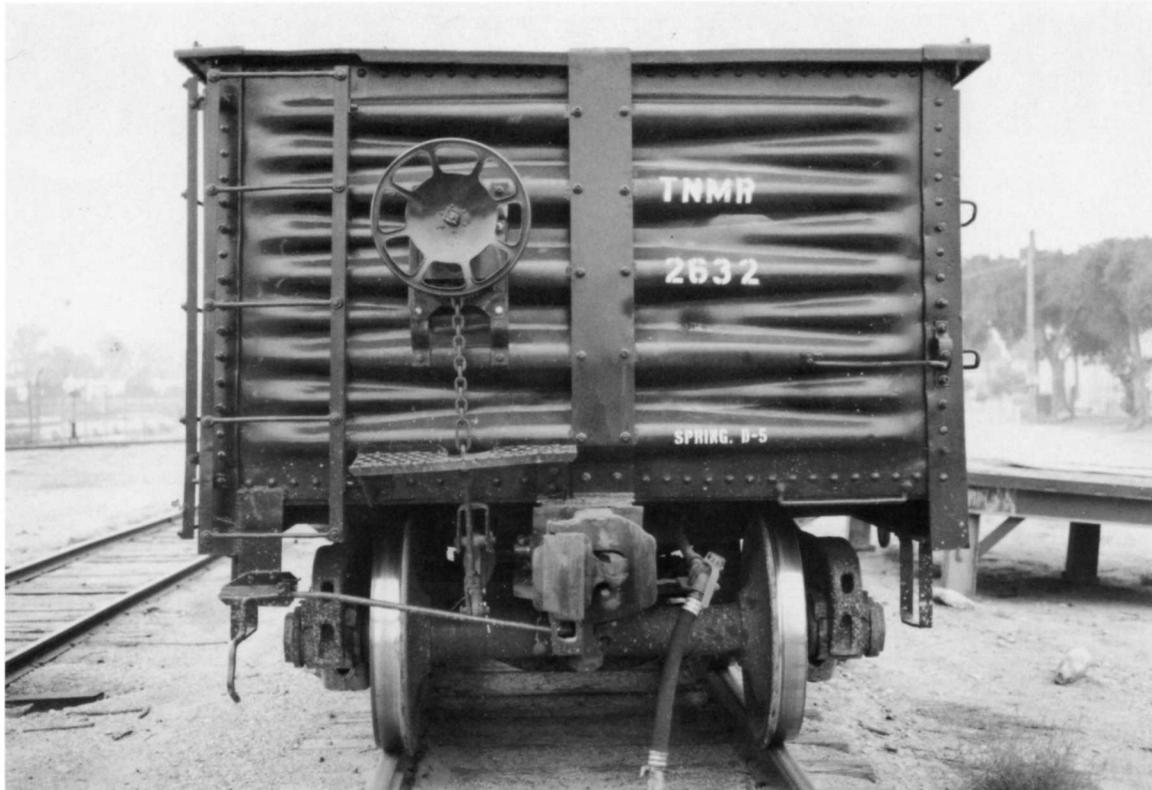
**TNMR 2632 (Above).** End view detail. shows the five large double tapered corrugations with minor ones in between. The strap in the middle helps reduce end bulge. Note extensive riveting along bottom and sides.
