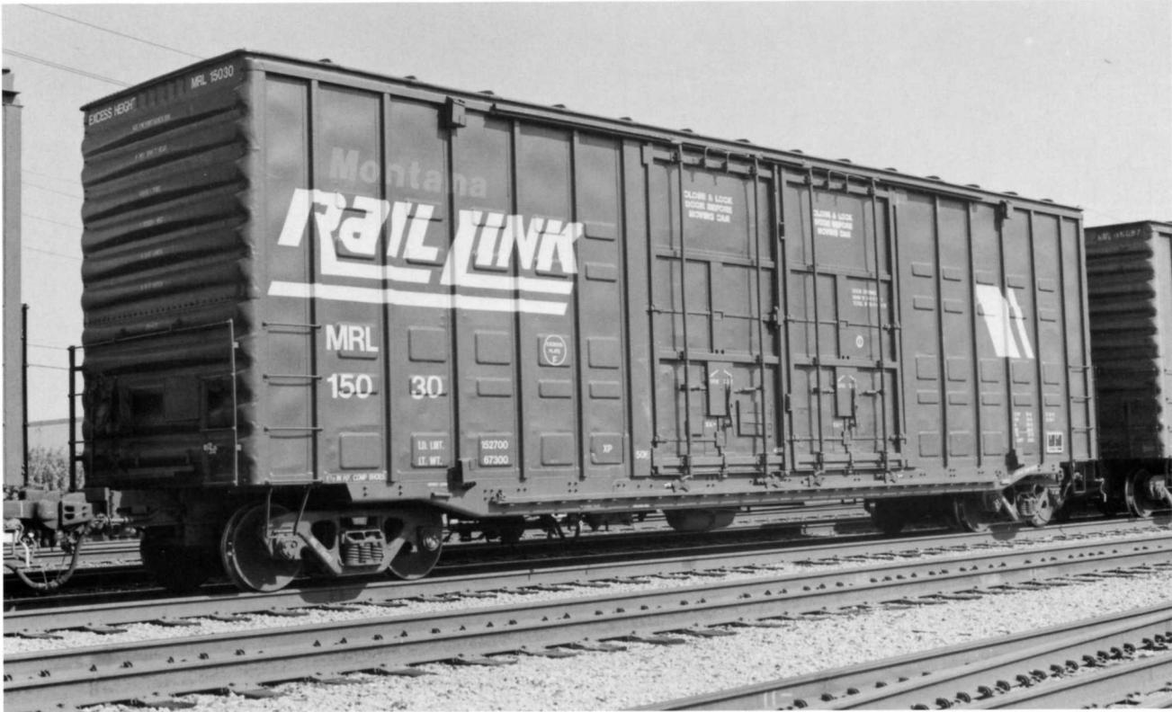
**MRL 15030** (Above) showing it in full MRL livery. Note the 2/4/5/ stamped corrugation end, flat roof and ten post side. These are only 70-ton cars so the load limit of this one is 152,700 lbs.
