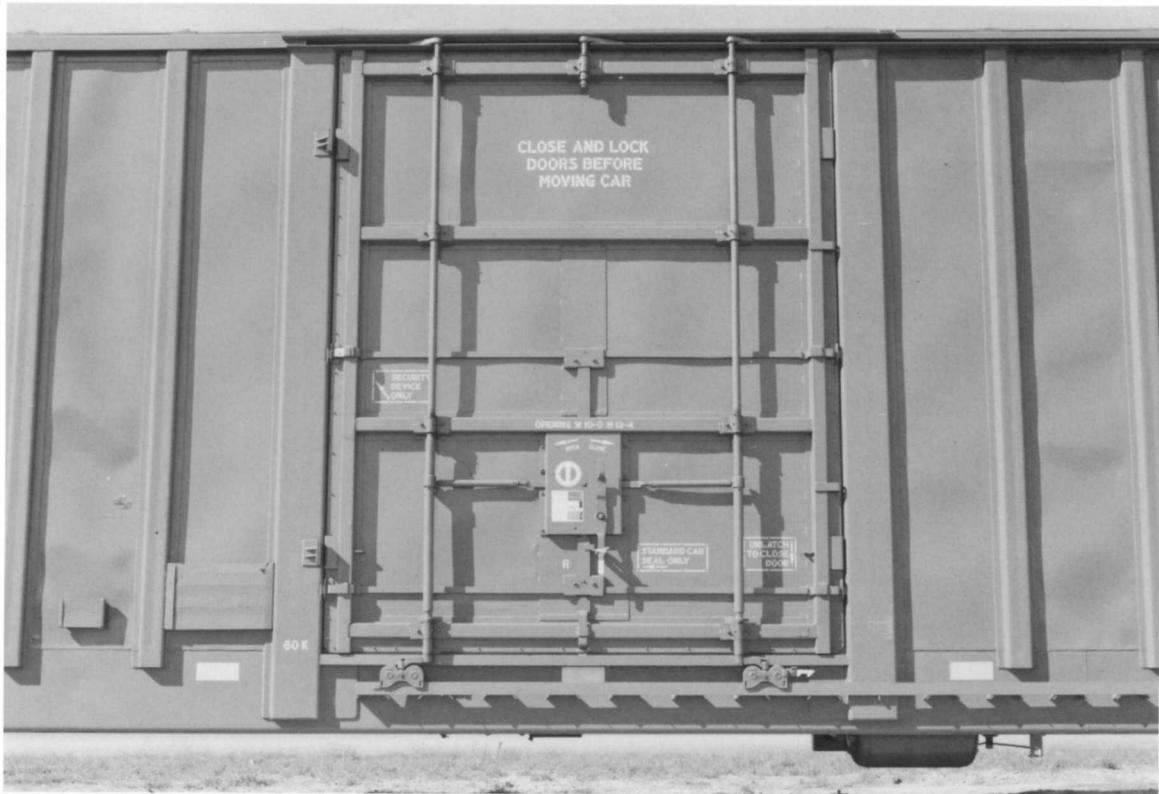
**BN 286157.** (Above). Detail of door area. Note how narrow the door looks especially with the massive door frame.
