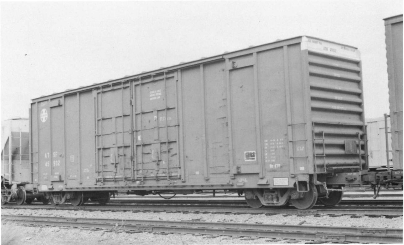
**ATSF 45932.** (Above). Pullman-Standard built 100 of these in 1974. These are 50'6" IL Plate F box cars. Door opening, 16'0" x 12'0" (WxH). Santa Fe class, Bx-170. Series, ATSF 45900-45999. Note the four wide side posts (ribs) to either side of doors. Pullman-standard rolled 3/3/5 ends. Flat roof. Cubic-foot capacity, 6196.
