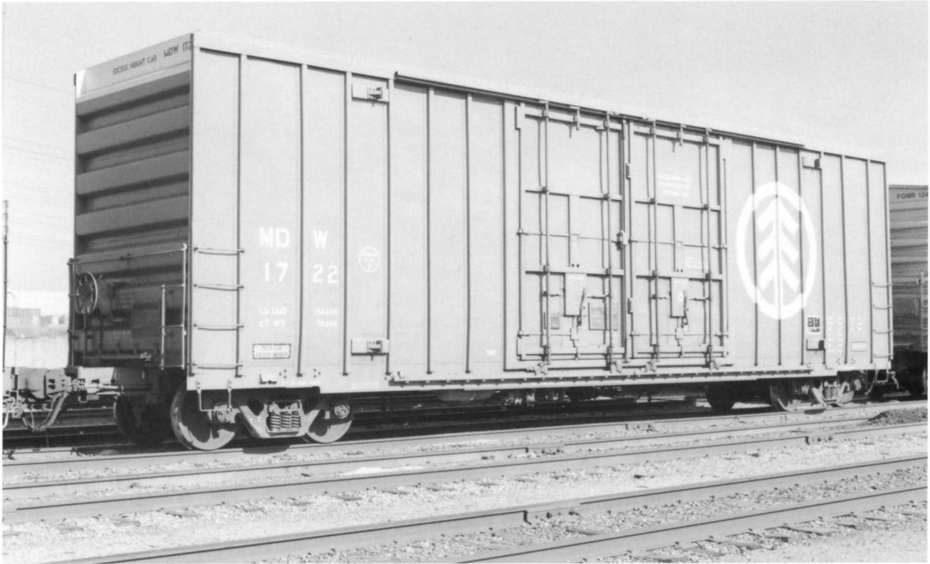
**MDW 1722.** (Above). This is a 50'6" IL Plate F box car. Door opening is 16'0" x 12'0" (WxH). Series MDW 1700-1799. The correct stencilled cubic-foot capacity is 6,241 (Registers list it as 6,246). This car was built in July 1976. Note flat roof, 2/2/3 corrugated ends and twelve post sides.
