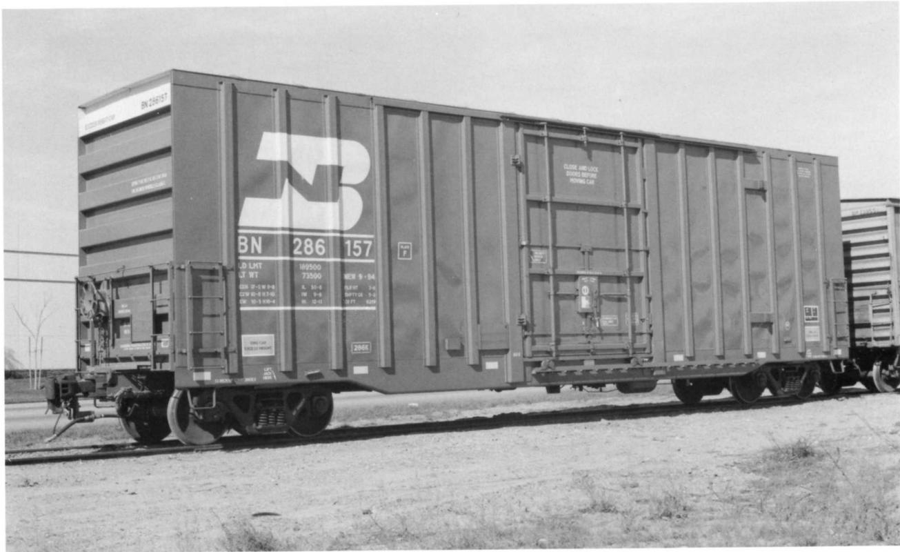
**BN 286157.** (Above). National Steel Car (Canada) built 150 of these for the BN in 1994. These are 50'6" IL Plate F box cars. Note the relatively narrow 10'0" x 12'4" (WxH) plug door. Note the 1/2/2 corrugated end, flat roof and twelve post side.
