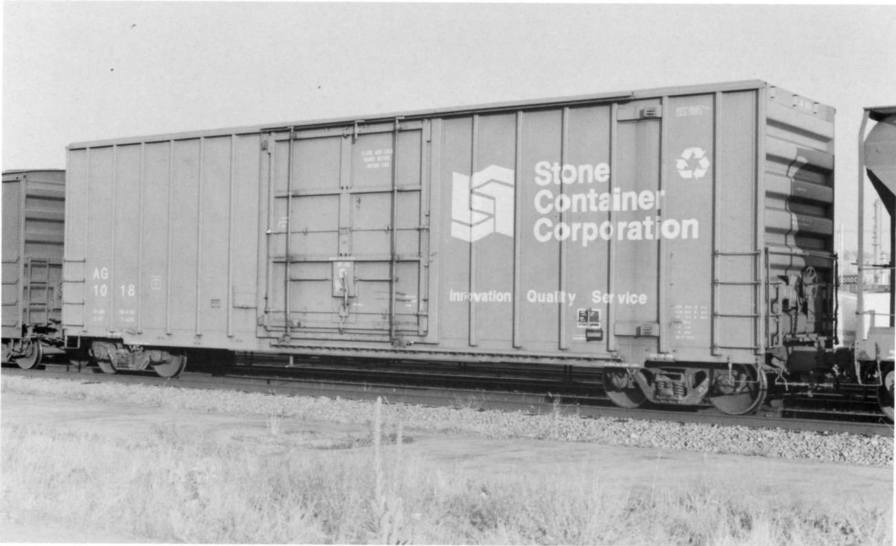
**AG 1018.** (Above) Gunderson built 50 of these for the A&G Railroad (Alabama) in 1990. Series, AG 1000-1049. Correct stencilled capacity is 5,757 cubic-foot (Registers show 5,505). Door opening, 12'0" x 12'0" (WxH). This car was built before Gunderson went to a wide side post. Note the 2/2/3 corrugated end, flat roof and twelve side posts.
