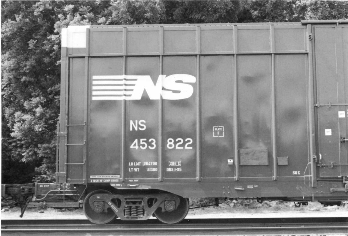
NS 453822 (Above). Left side detail. Note the 286K GRL stencil and the load limit is correctly matched at 204,700 lbs (the load limit plus the light weight will total 286,000 lbs).
