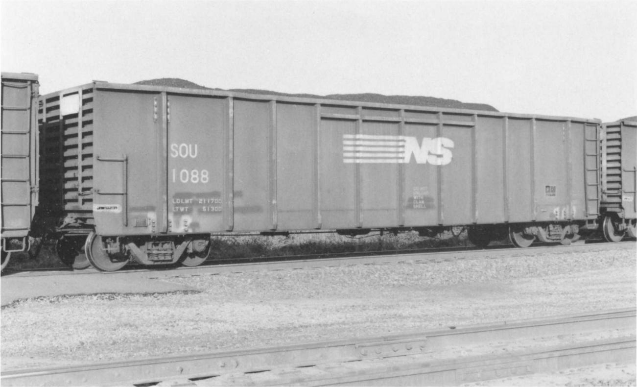
**SOU 1088.** (Above). Certainly one of the first aluminum-bodied unit trains to be placed in regular service was the Southern 1000-1749 series. The cars were built in 1960 by Pullman-Standard's Bessemer, AL plant. Each car had a whopping 3,620 cubic-foot capacity. NS class GS-1. The warning in the center says...Do not unload with clam shell.
