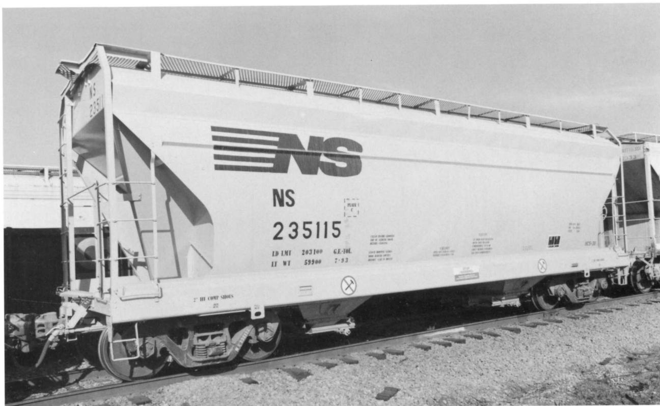
**NS 235115.** (Above). Originally built for Southern as series 91000-91599 by ACF's Huntington, WV plant. This is a 3,300 cubic-foot capacity ACF Center Flow®. It was repainted in July 1993 by GE's Toledo shop. NS class HCS-38.
