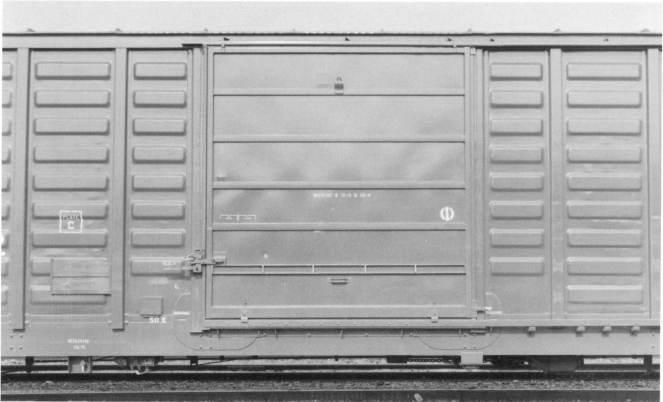
NS 41112. (Above). Center section detail view. New sliding doors replaced worn-out originals as cars were refurbished. Markings indicate 50,000 lb capacity nailable steel floor.
