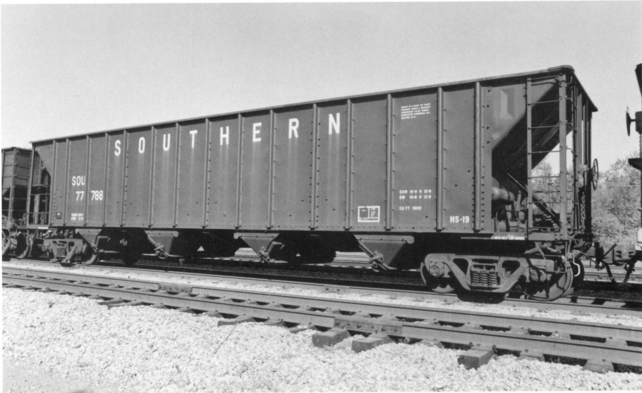
**SOU 77788.** (Above). Built in 1971 by Greenville Steel Car as part of Southern's 77200-77799. Norfolk Southern's influence is shown here with the repaint and new class HS-18. These are 3,600 cubic-foot capacity quadruple hoppers used for coal transport. Photographed in Birmingham, AL May 1994.
