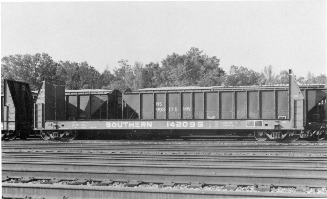
**SOUTHERN 142095.** (Above). Still in original paint as delivered from the builder (Greenville Steel Car) in July 1980. This is a 50-foot Plate C pulpwood car. Series, Southern 141300-142099. The remaining cars would become NS class FS-95 after the merger. Photographed in Crewe, VA during May 1995.
