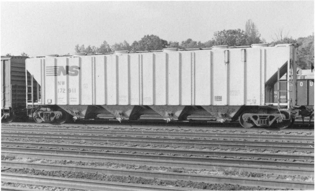
**NW 172911.** (Above). This huge 100-ton 5,200 cubic-foot capacity covered hopper was built in 1967 by N&W's Roanoke, VA shop. Series, NW 172900-172999. N&W/NS class HC-65. Photographed in Crewe, VA during May 1995.
