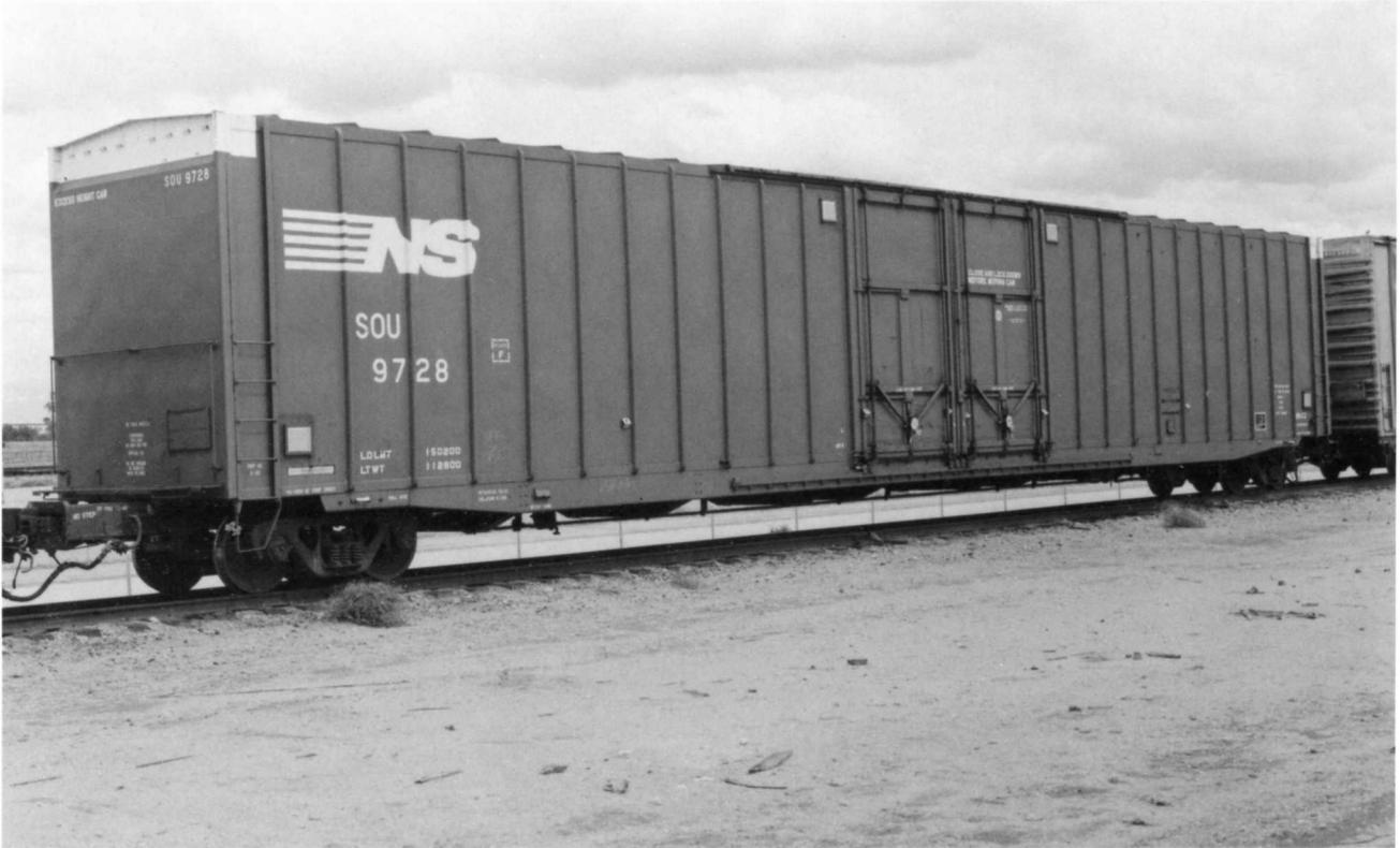
**SOU 9728.** (Above). Southern had some very interesting freight cars - none the least is this 84'4" IL Plate F+ double-plug door box car. The car has a 10,036 cubic-foot capacity, 75-ton load limit (on 100-ton trucks) and is equipped with Pullman's very own 30 inch cushioning device.
