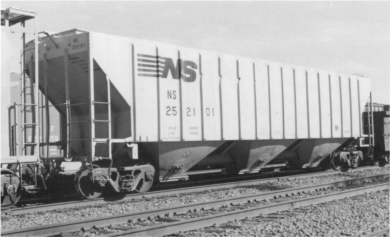
**NS 252101.** (Above). Pullman-Standard built 1,000 of these 4,740 cubic-foot capacity covered hoppers in 1969 for the N&W. Originally part of the series NW 173000-173999. The series is now 252000-252901.
