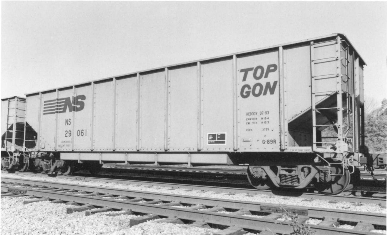
**NS 29061.** (Above). Norfolk Southern began converting a number of old coal hopper into coal gondolas by replacing the original hopper body with a new gondola body. This one was rebodied in July 1993 by the NS Roanoke, VA shops. The cars are gray with black lettering. Photographed in Birmingham, AL during May 1994.
