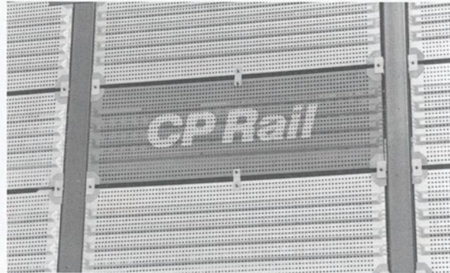
Fig 20. CP Rail's white on perforated/corrugated red panel.
