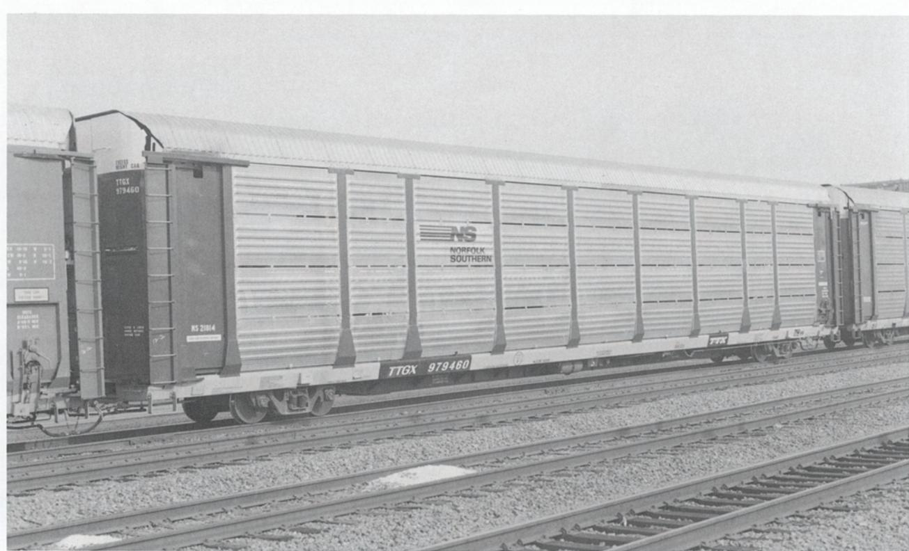
**Fig 11.** (Above) Norfolk Southern's NS 21814 on TTX 979460. The B3 panel on this rack is solid/corrugated and remains in natural metal color with a black NS logo. The rack structure is brown and white.
