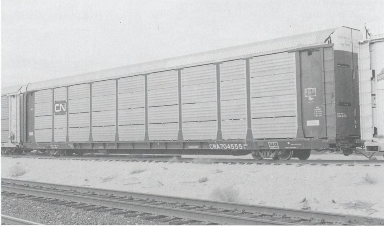
**Fig 3.** (Above) Canadian National's CNA 704555 is black with white data (and of course natural metal panels). The CN "noodle" logo appears in the B2 position. The "2" nd "8" position panels are the smallest.
