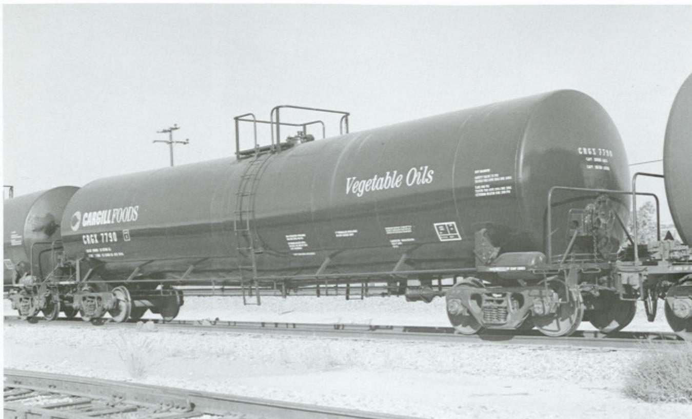
(Above) **CRGX 7790** is part of a 250 car order built October through December by Trinity's Longview TX plant. Notice the new Cargill livery with no less than three different styles of lettering! The Cargill logo is green (and black). The 25,500 gallon cars are used for vegetable oil transport. Series is CRGX 7640-7889.
