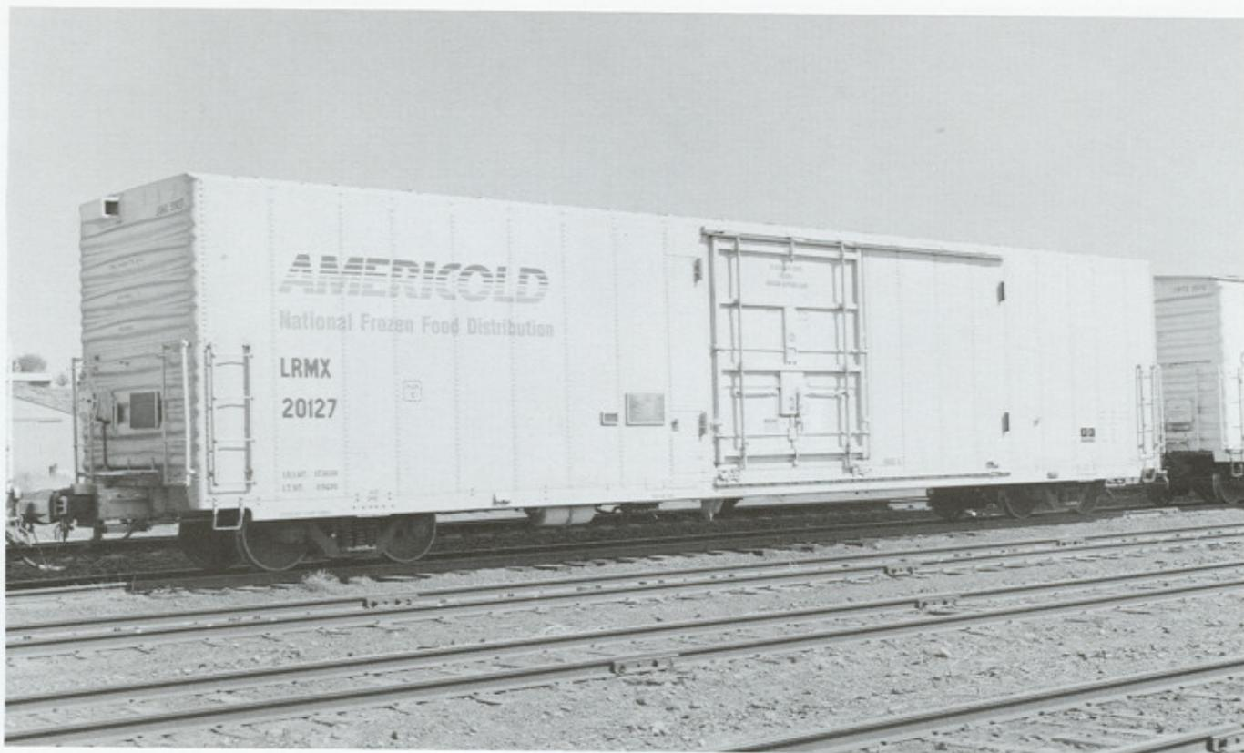
(Above) **LRMX 20127** is a cryogenic refrigerator car (AAR, RC) that was acquired by Logistics Resource Management in 1994. The cars are owned by Greenbrier Leasing. Series is LRMX 20120-20129.
