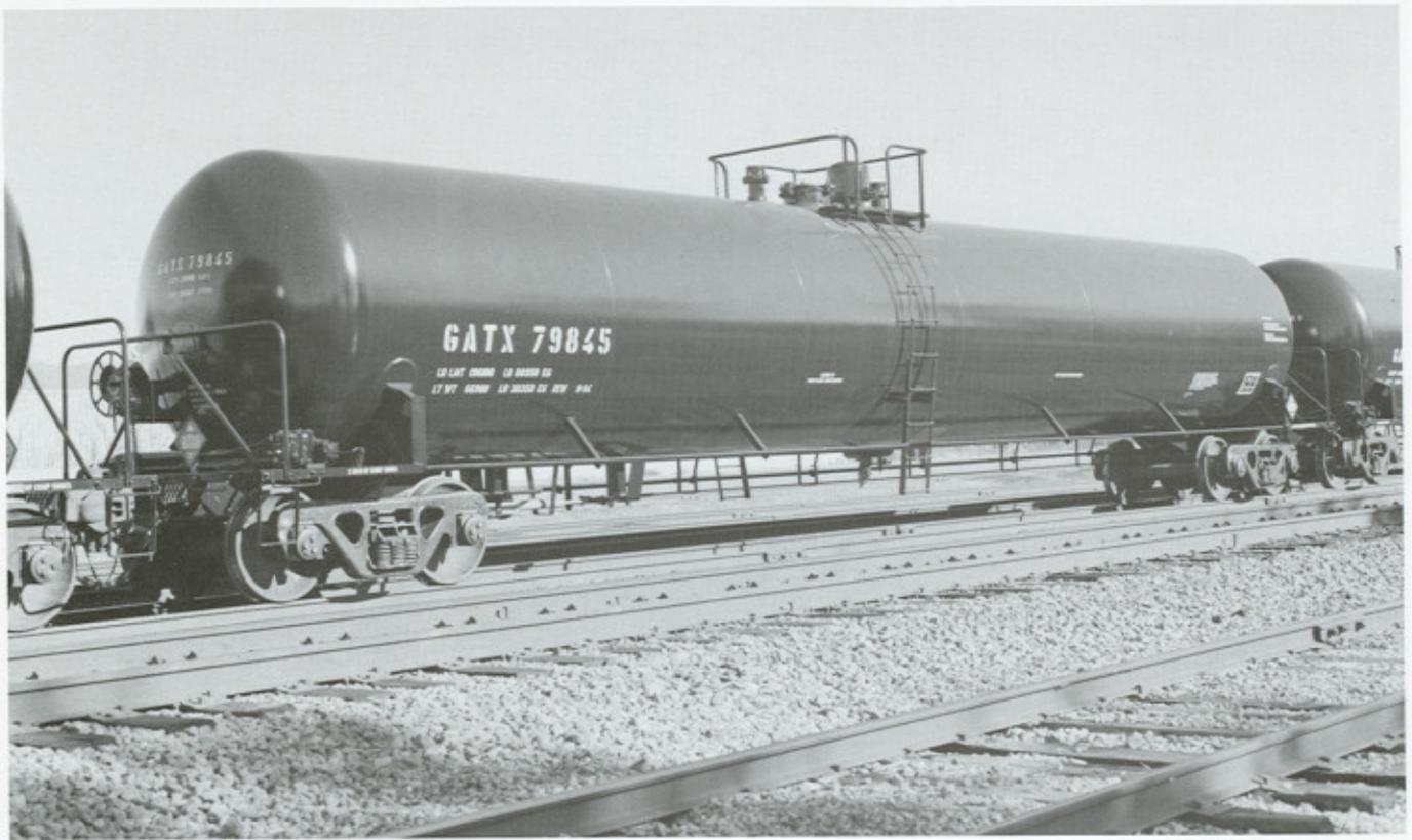
(Above) **GATX 79845**. This car was built in November 1994 by Trinity's Longview, Texas plant. These are 30,000-gallon non-insulated un-coiled 111A100W1 tank cars used for transporting alcohol. There are 85 cars in the series GATX 79842-79926.
