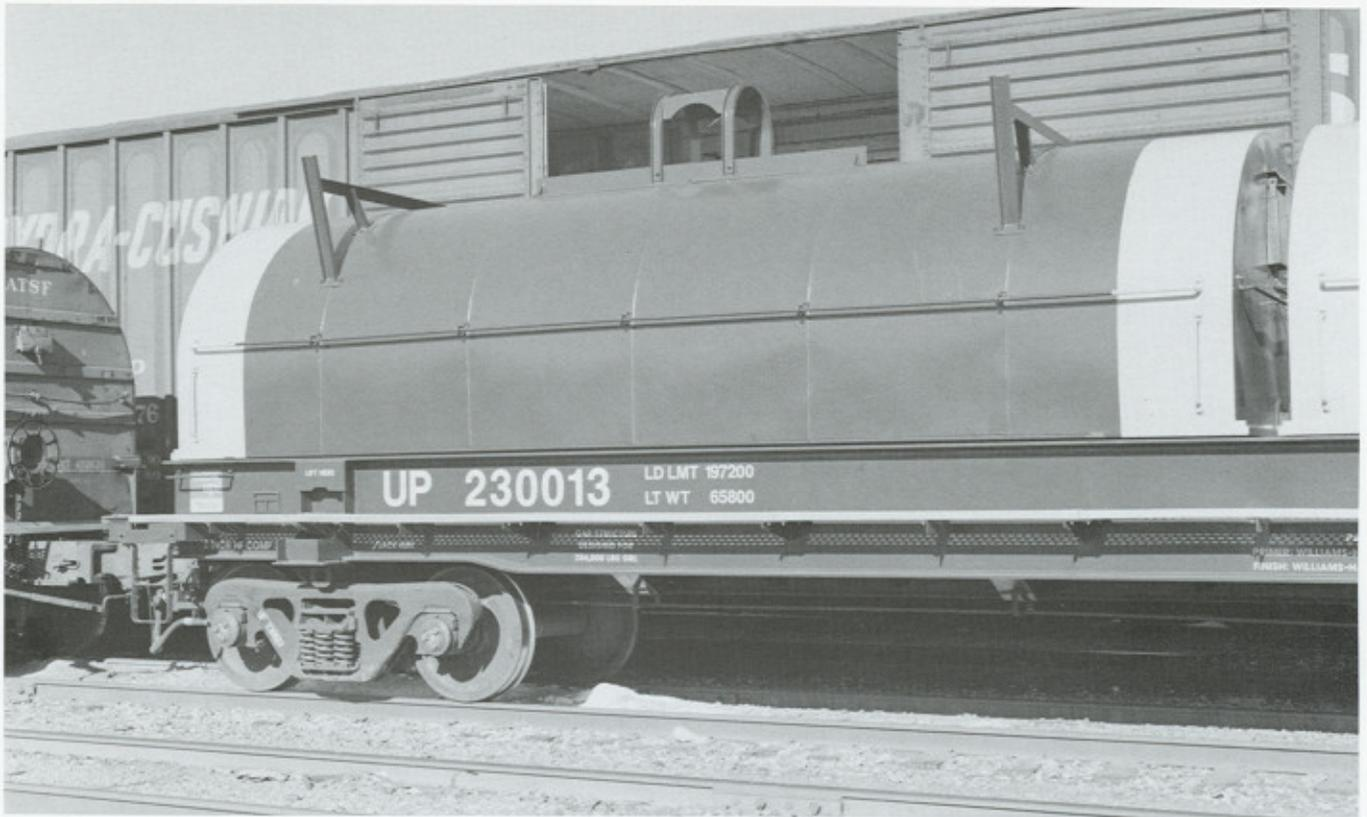
(Above) Left side detail of UP 230013. Notice the load limit of 197,200 lbs. However, right below it is a notice indicating a 286,000 lb gross rail loading (GRL). Note that even the traditionally CSX-ish *Ease Up!* stickers are present.
