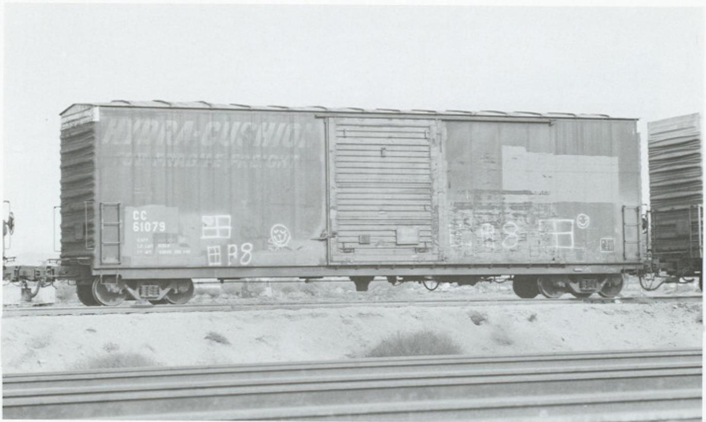
(Above) **CC 61079** is part of a group of 88 cars transferred to the Chicago Central & Pacific in 1994 (numbered CC 61001-61088). The cars were originally built for the SSW/SP as part of class B-70-32 in 1967. The 50'5" IL Plate F single 10'6" sliding door box cars are being used in appliance service by the CC&P. Shown here in December 1994.
