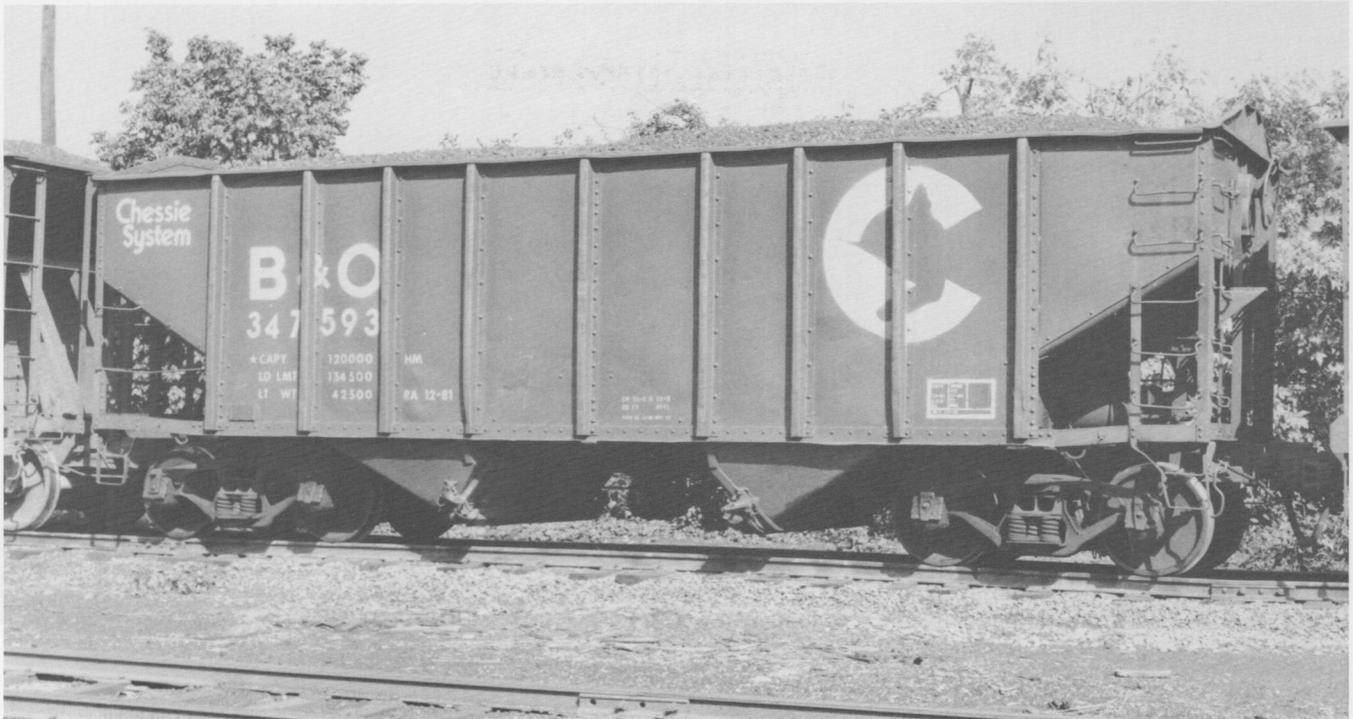
(Above) B&O 347593 photographed at Huntington WV in September 1985. Still in pretty good shape for forty years of service! Built 12-46. 2141 cf. It's ex C&O 347593, rebuilt from an offset-side car in 1963 (nee from C&O 47500-48989). (Below) IHB 7746 was ADN 7746 built by USEX. Photographed at Mira Loma, CA in April 1991.
