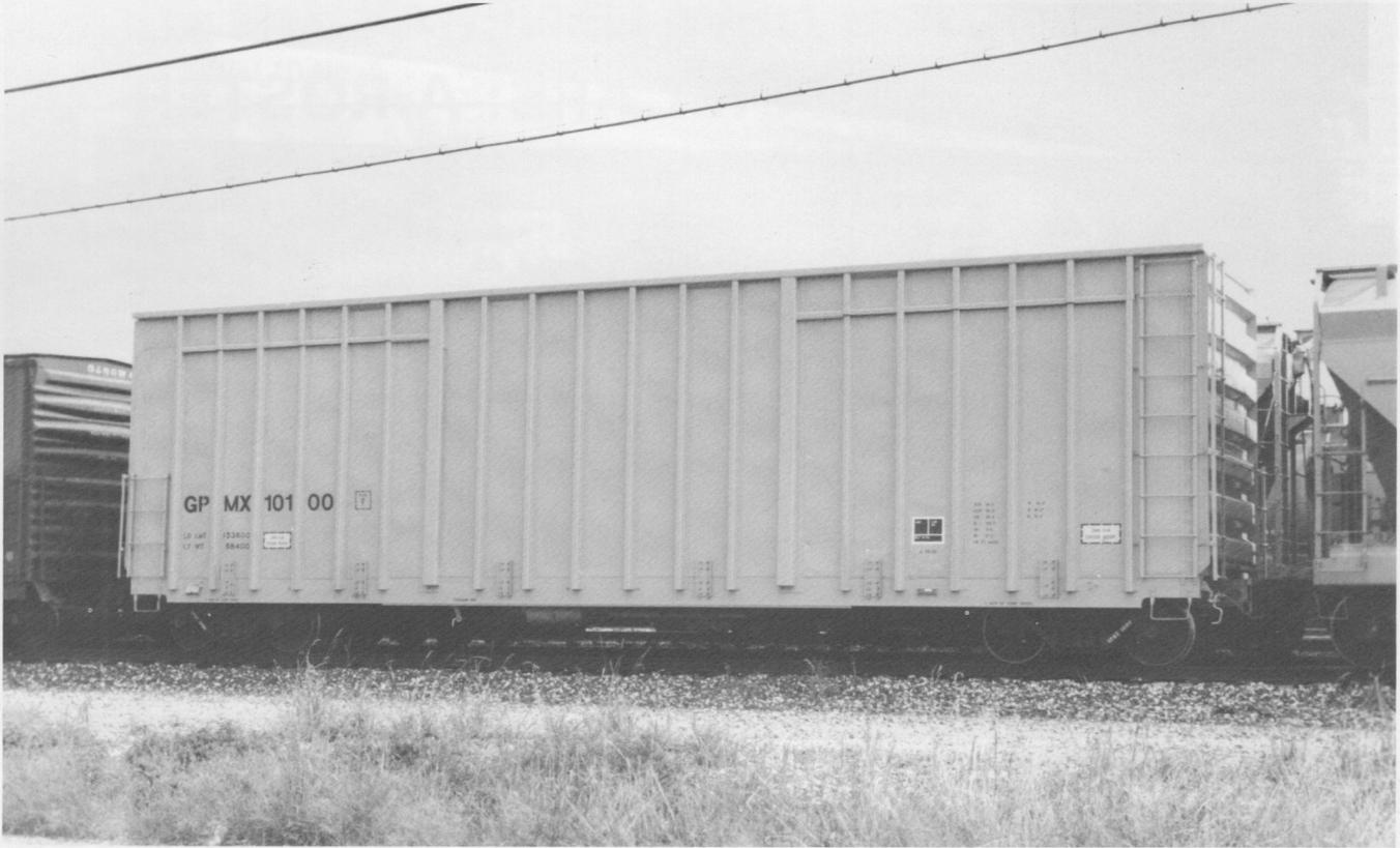
(Above) GPMX 10100, overall view. This car was converted from a SP class B-70-73 box car to a Plate F gondola car. (Below) "B" end view detail. Note the end ladder to the left of the brake wheel.
