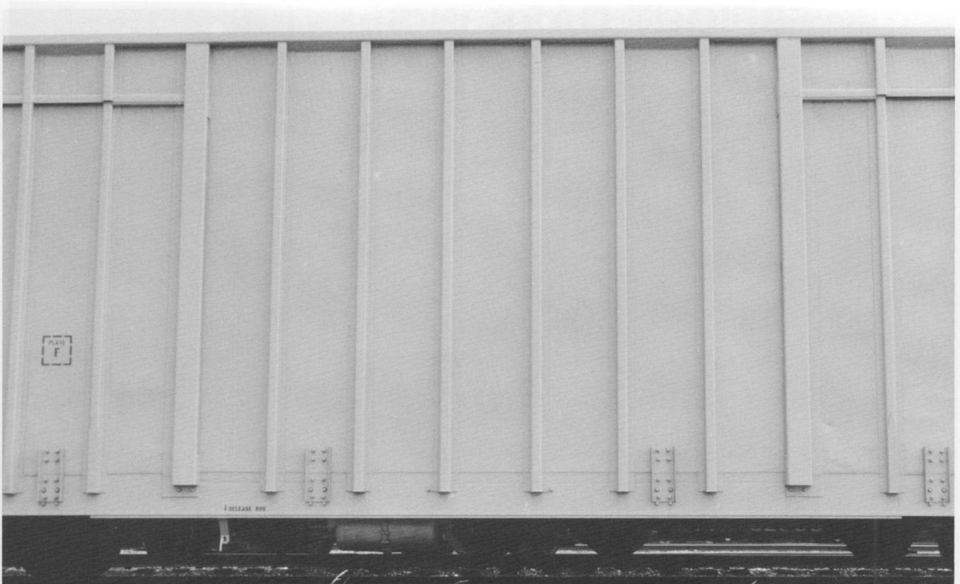
(Above). Center section detail. Channels were added for lower side reinforcement. The area between the wider ribs appears to be the previous location of the door opening. (Below) "A" end detail view. The cars has a 6028 cubic foot capacity. Note the FMC side sill design from the box car.
