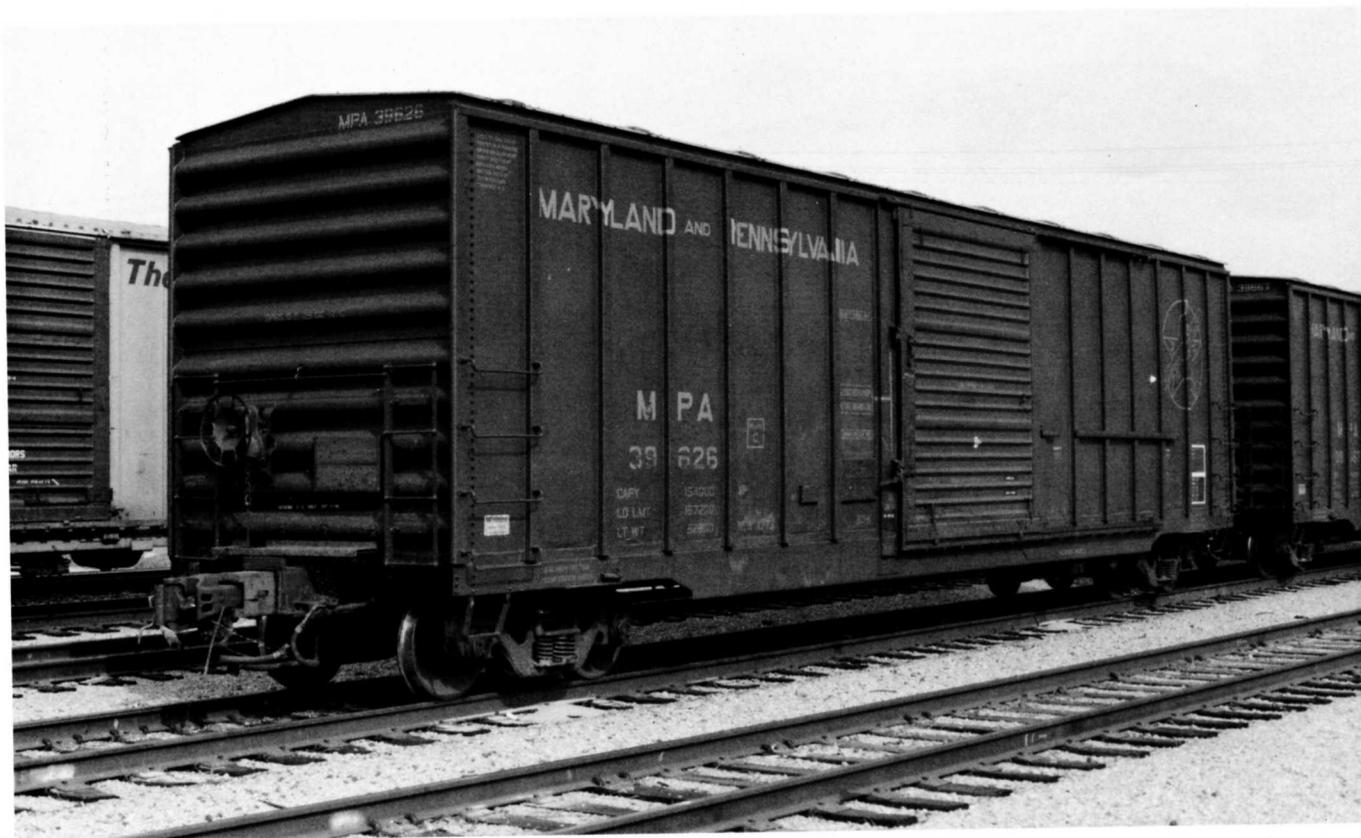
(Above) MPA 39626 built was in 1979 as part of Lot 41800. This series came equipped with 15" end-of-car cushioning. (Below) NW 604515 was built as part of Lot 37700 in 1979. These fascinating 60-foot 100-ton Plate F+ box cars were used in auto parts service by many railroads. Both photos by David G. Casdorff.
