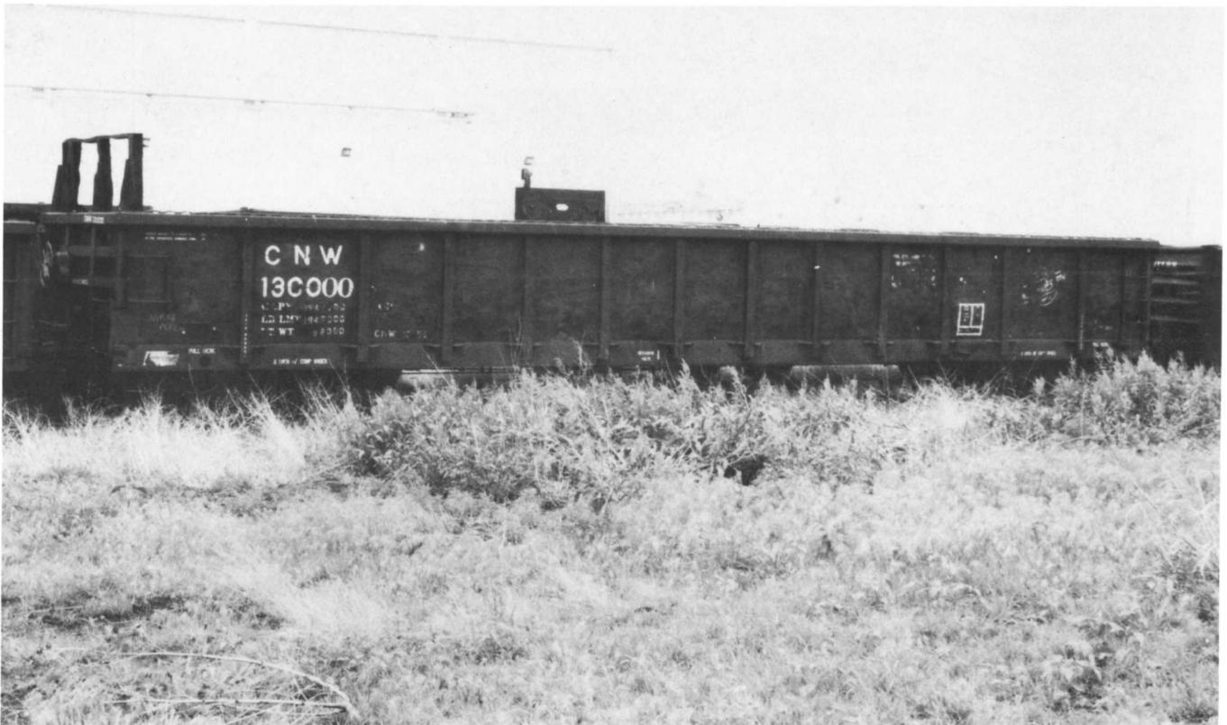
(Above) CNW 130000, the class car of the 130000-130299 series (SIECO ATL, 5-80). What's left of one of the bulkheads can be seen at the left end of the car. Note that the last two "00" digits have a different style than the rest. This car also has a continuous tie down rod (not used very often in scrap service). May 1991. (Below) CNW 340016. This car illustrates the height difference between the 2244 and the 2493 cuft cars (note CNW 130000, on right). May 1991. Both photos by James Kinkaid.
