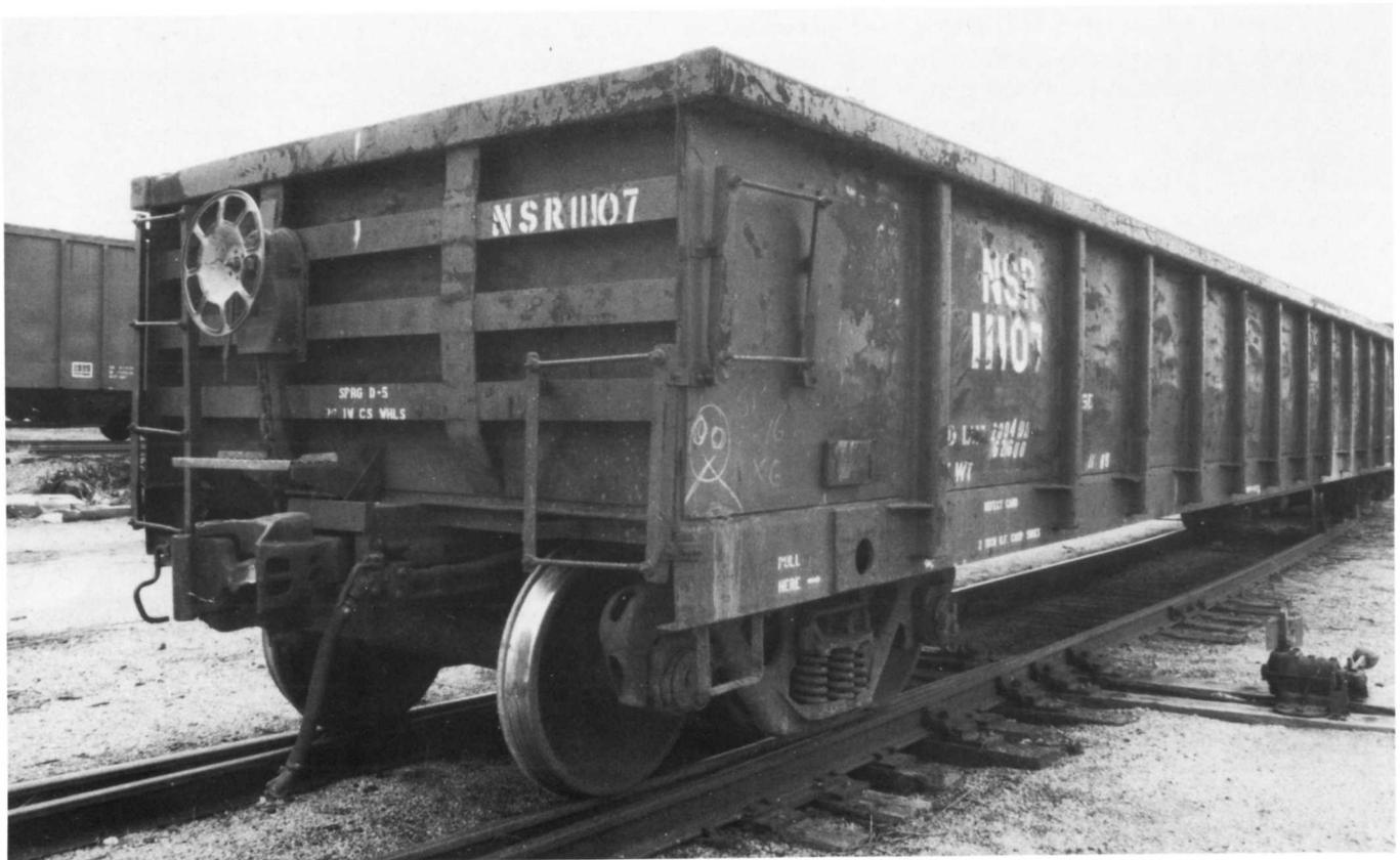
(Above) NSR 11107, "B" end view. Of particular note are the vertical stiffeners which are bent in at the bottom. Also note the heavy demarcation line between the car side and the lower side channel. (Below) NSR 11107, "A" end view. Of particular note here is how the 6"x6" top chords project out past the car ends. Note also the "2240" cuft capacity markings. Both photos by James Kinkaid.
