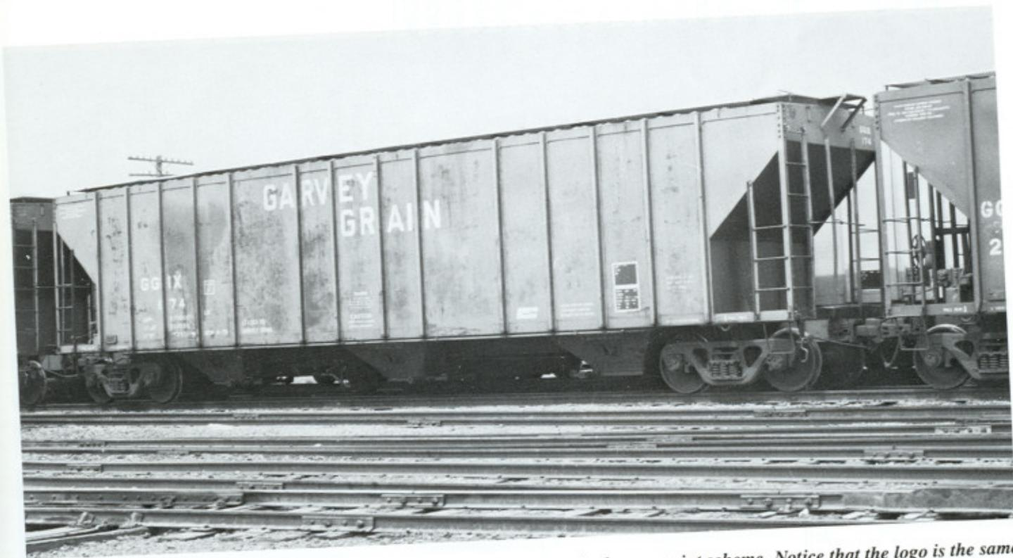
*GGIX 174. Although getting a little ragged, this car illustrates the standard green paint scheme. Notice that the logo is the same style as is on the orange cars. Also note how the car top stiffeners are so visible, even from ground level. September 2, 1990.*
