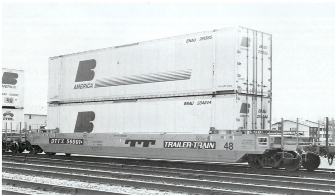
*DTTX 56001 is one of 150 single-well double stack container cars ordered from Gunderson by Trailer Train. M.B. Foley.*
