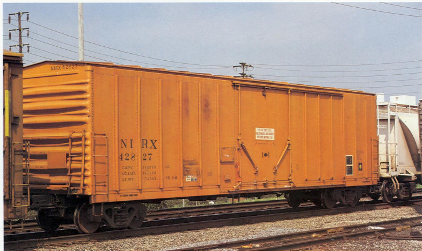
*NIRX 42827 is shown here on June 3, 1983 leased to Pfizer. This is a 70-ton RBL (despite the incorrectly applied LO mechanical designation!)*
