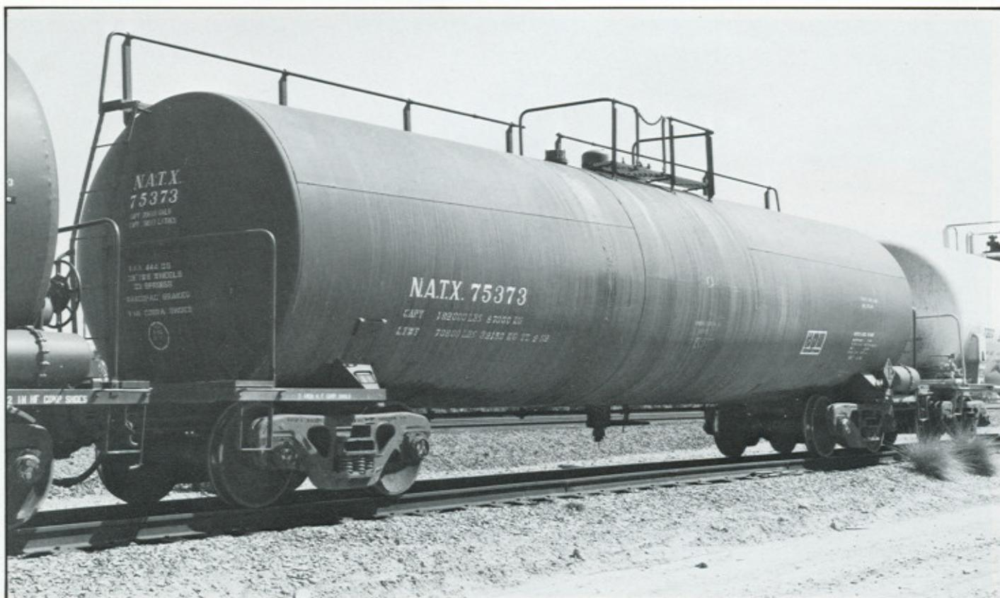
*NATX 75373 was built in 1974 and is a 20,600-gallon, 100-ton, general-service insulated tank car. Lessee is Borden Chemical. Note the uncommon (for this size tanker) full length top walkway.*
