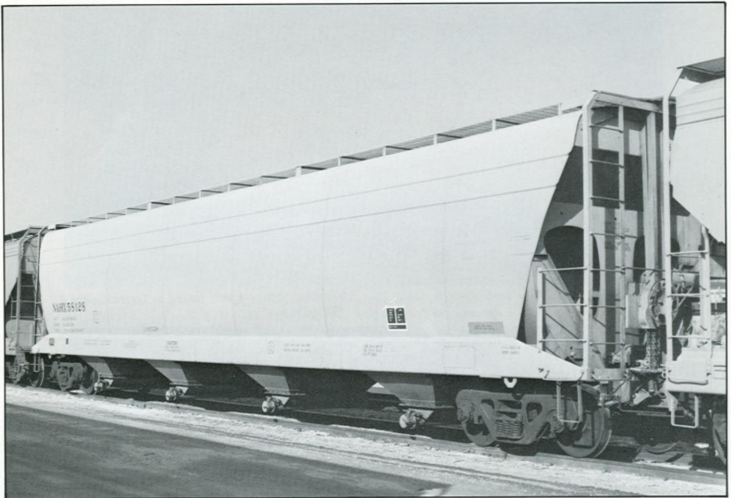
*NAHX 58128 was built in September 1973 by NACC's Texarkana shops. It is a NACC 5852-cuft design covered hopper. Note the sharp angles on the ends of the side that readily distinguish this NACC design family.*
