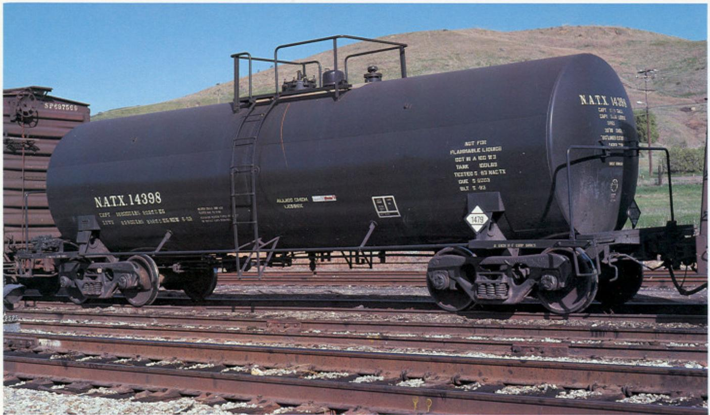
*NATX 14398 was one of the last tank cars to come off the Texarkana assembly lines. Shown here on December 25, 1984 in San Luis Obispo, CA. It was built in May 1983 and is leased to Allied Chemical. It is a 100-ton, insulated, coiled, tank car. Pat Holden photo.*
