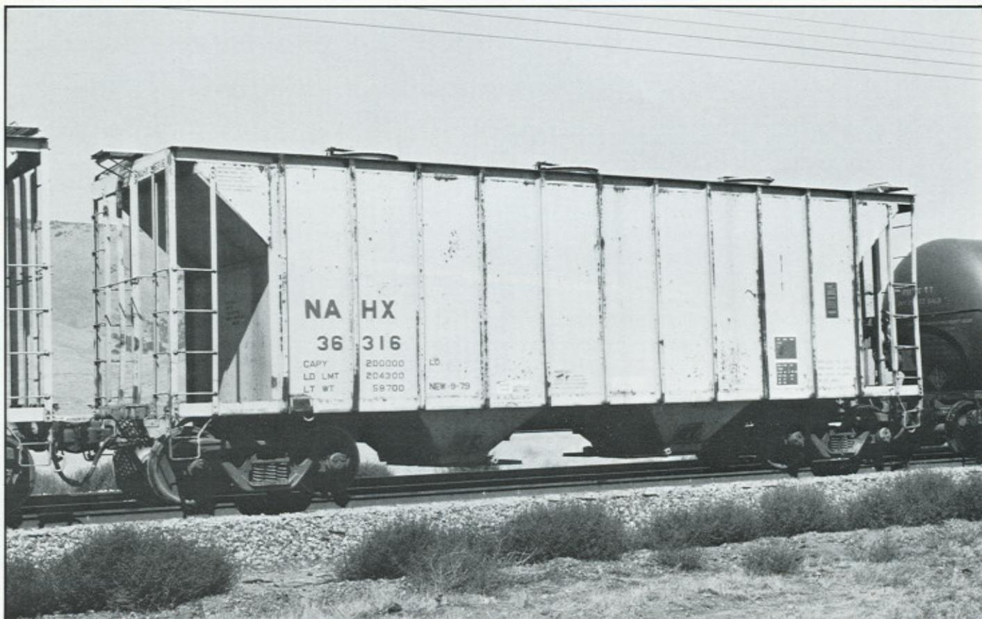
*NAHX 36316 was built in September 1979 by Greenville Steel Car. It is a 100-ton, two-bay covered hopper. GSC 2917-cuft design.*
