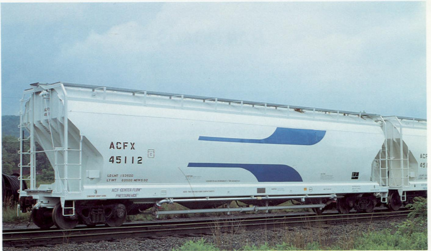
ACFX 45112 was built by ACF in May 1990 for lease to Allen Bradley/TDK Magnetics. This is ACF's PD5000 Center Flow® covered hopper with the blue "wings" markings. E.A. Neubauer photo May 1990.
