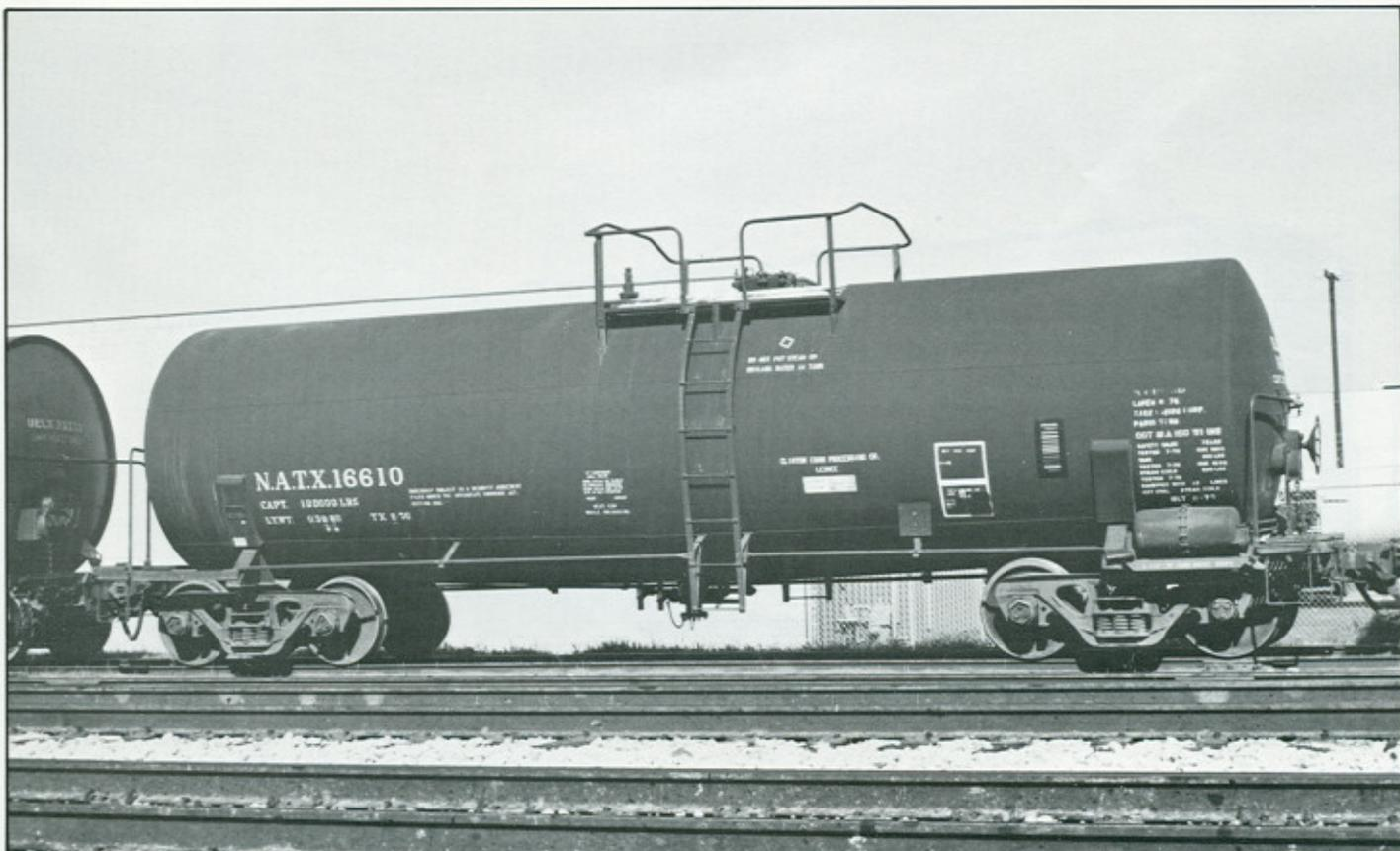
*NATX 16610 shows the offset inlet style of this series of tank cars (16210-16665) built at Texarkana. This car was built in 1976 and is leased to Clinton Corn Processing Co. for corn syrup transport.*
