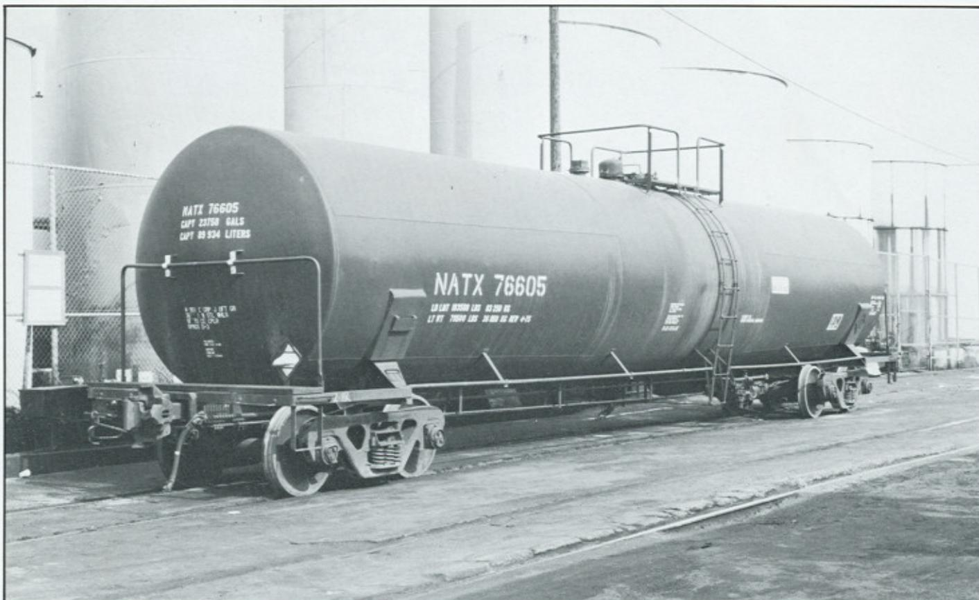
*NATX 76605 is an insulated, coiled, 100-ton, 23,750 gallon general-service tank car leased to Exxon Chemical Americas. The car was built in April 1975.*
