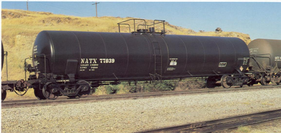
*NATX 77039 was built in June 1978. It is insulated, coiled and has top unloading only. Lessee is Rohm & Haas. Pat Holden photo, April 1986.*
