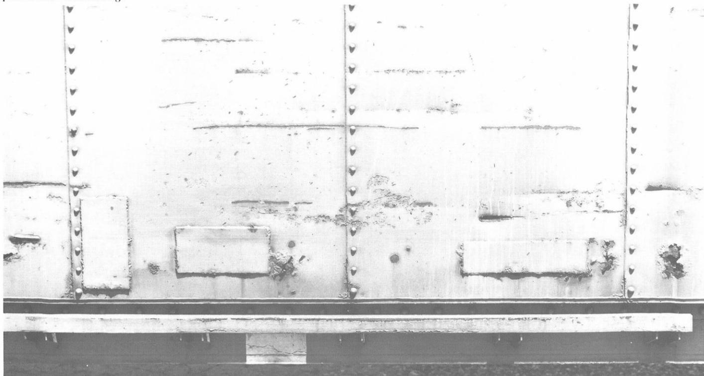
Interior post, double sheath, and insulated box cars often rust out or get punctured sheathing. Here is an example of repairs done to an RBL’s side sheathing. Note they are just rectangular patches welded on over the rusted or punctured area. The one on the left is about 4” wide by 12” tall, but they can be made for any size.
