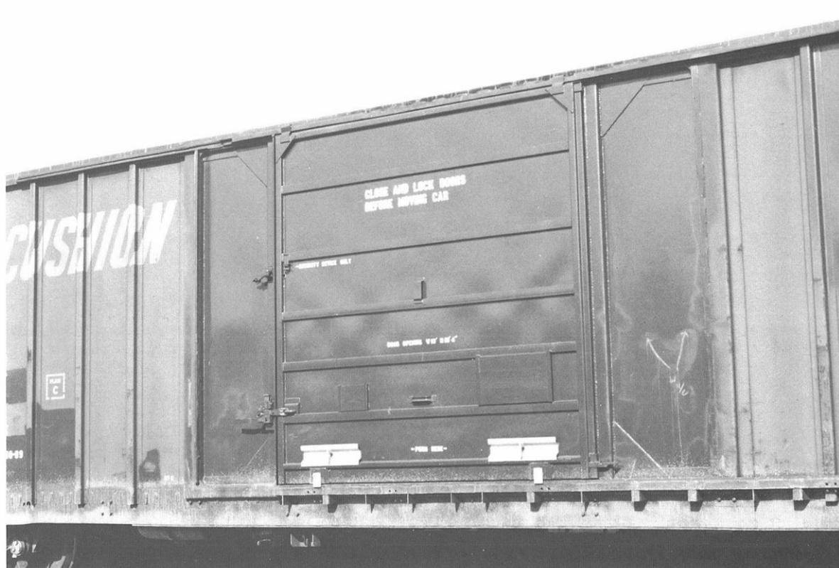
*A close-up of WCTR 66505's door area as viewed from the outside shows the area where the new 10-foot door replaced the former double 8-foot doors.*
