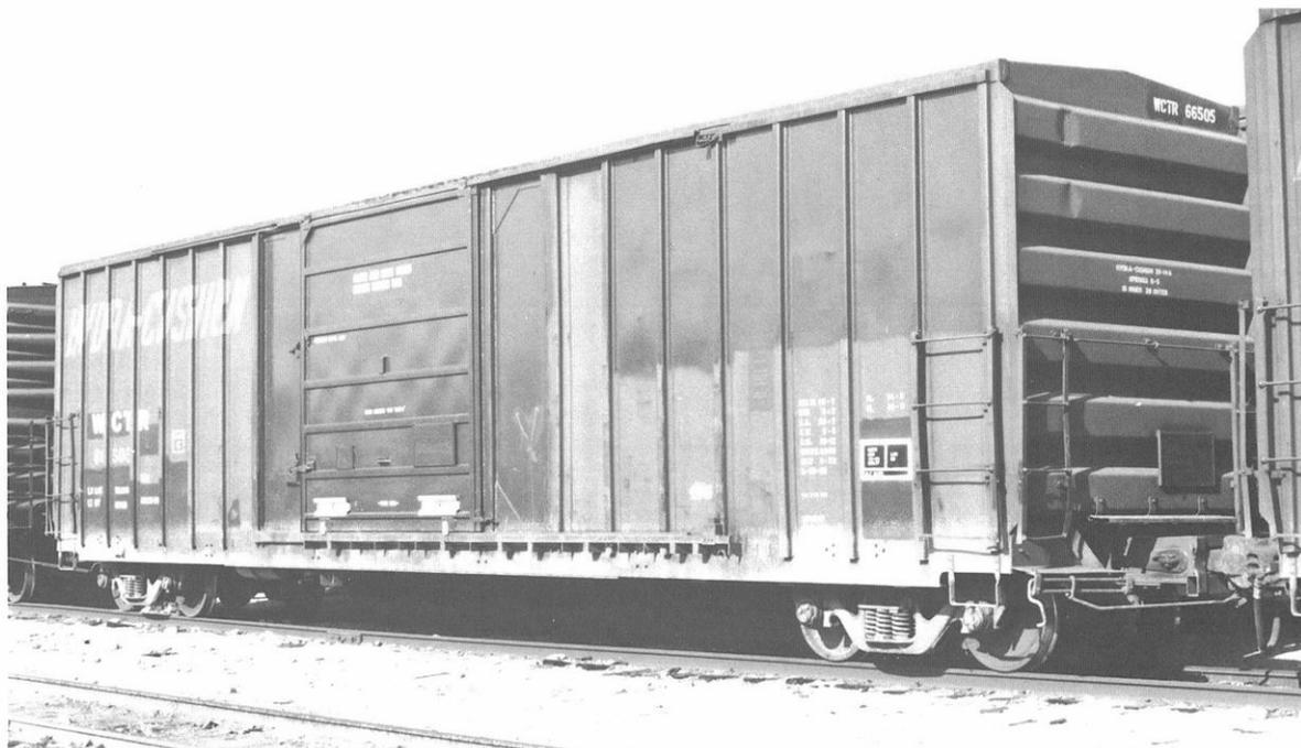
*WCTR 66505 was formerly SSW 66505 a double sliding door 50'7" box car. In this photo one can easily see the result of the conversion by the newly painted areas.*
