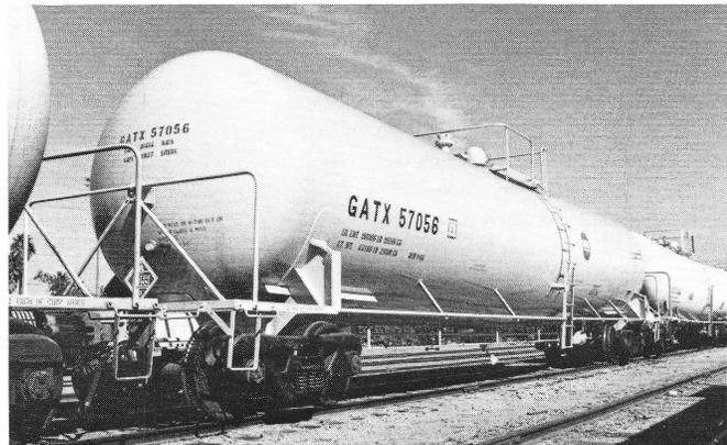
GATX 57056 is part of a new series of 26,500 gallon tank cars being leased by Dow Chemical. This car was built by Trinity in 9-88. The non insulated cars are being used for Aromatic hydrocarbon and styrene service. (David G. Casdorff)
