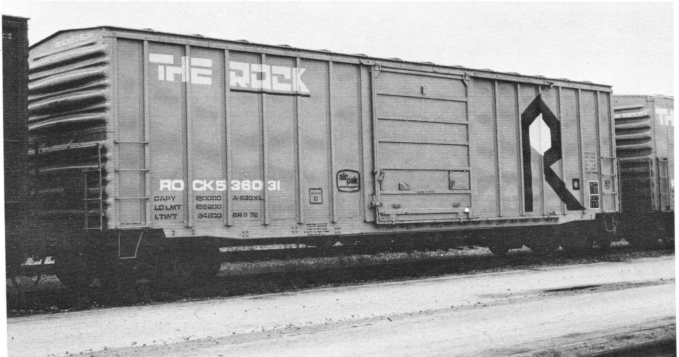
*ROCK 536031, makes a good prototype for the recently released McKean 50-foot outside braced ACF boxcar model in H.O. scale. The car comes from a series originally built in 1972 by ACF STL as RI 36000-36299. These were 70-ton loader equipped cars with a cubic foot capacity of 5285. (Pete Arnold photo)*
