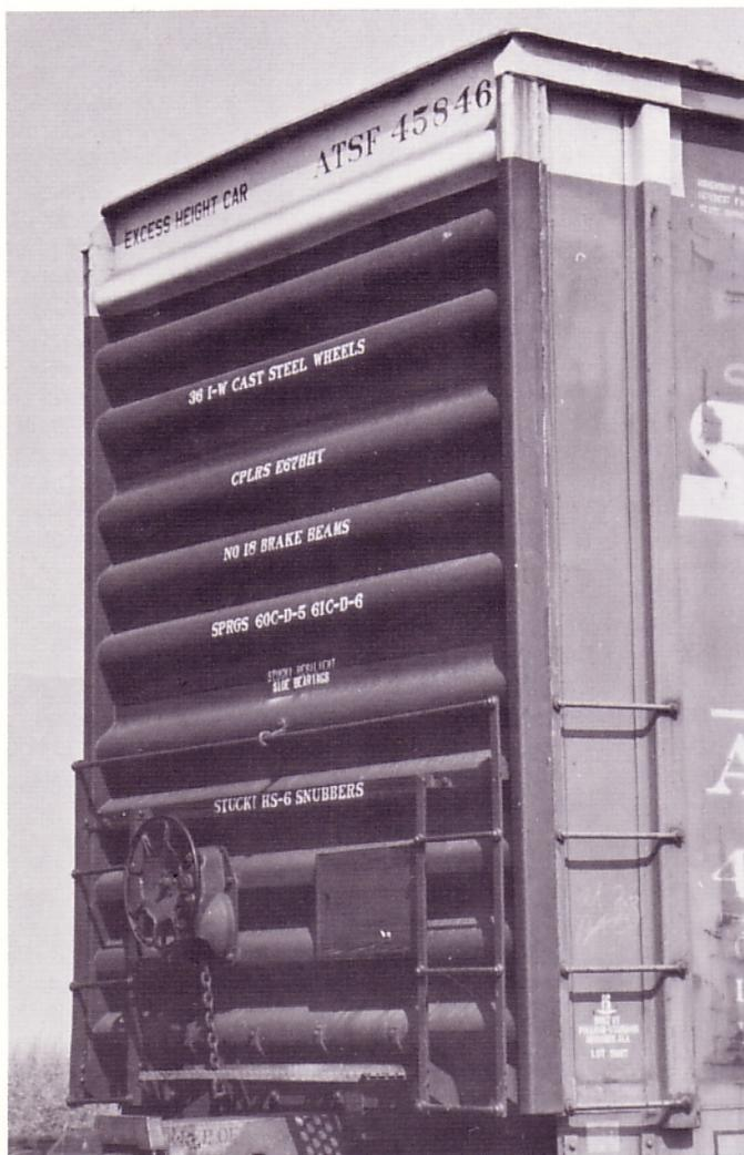
Looking now at the Pullman-Standard design end featured on both the BFF 6196 and PS 6196 designs. Note the "rolled" appearance of this design end. Also note welded seams in panels.
