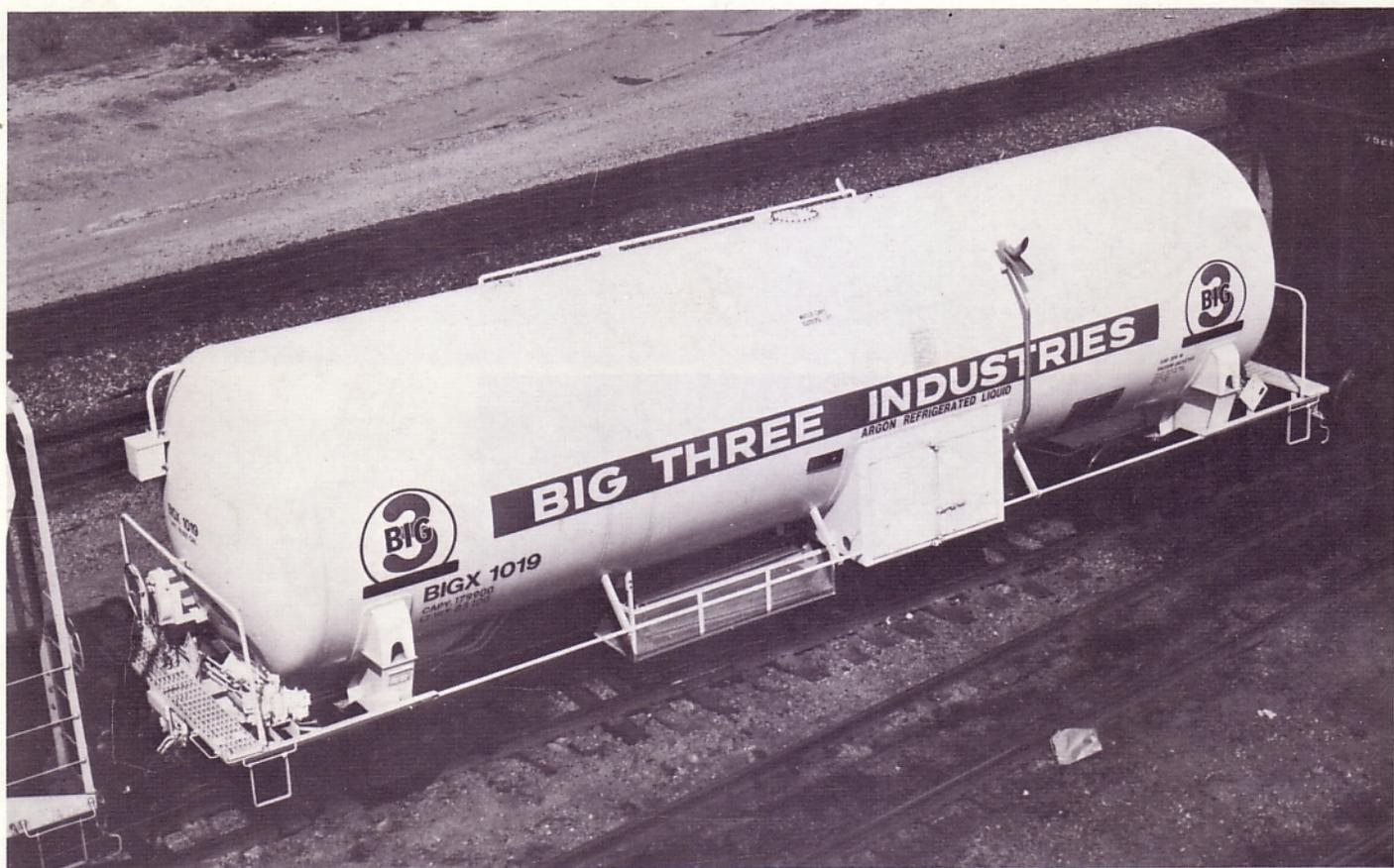
*BIGX 1019-1024. Built 3 = 5-85 by Richmond Tank Car, Houston, TX. These are probably one of the last tank cars built by RTC. These cars have a 16,555 gallon capacity.*
