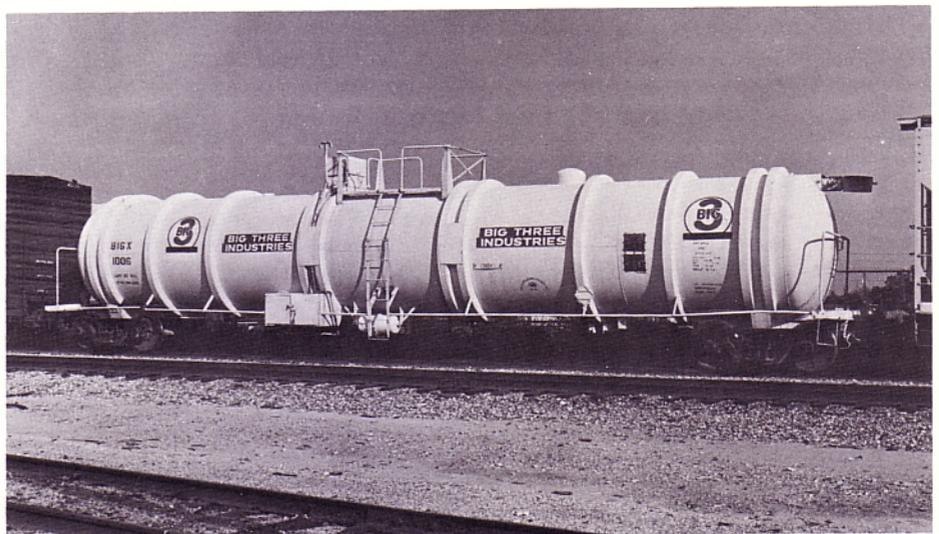
*(RIGHT) BIGX 1006-1011. Built 8-9-62, 11-63. This series has a 16,293 gallon capacity. These 100-ton cars are the oldest still on the fleet.*
