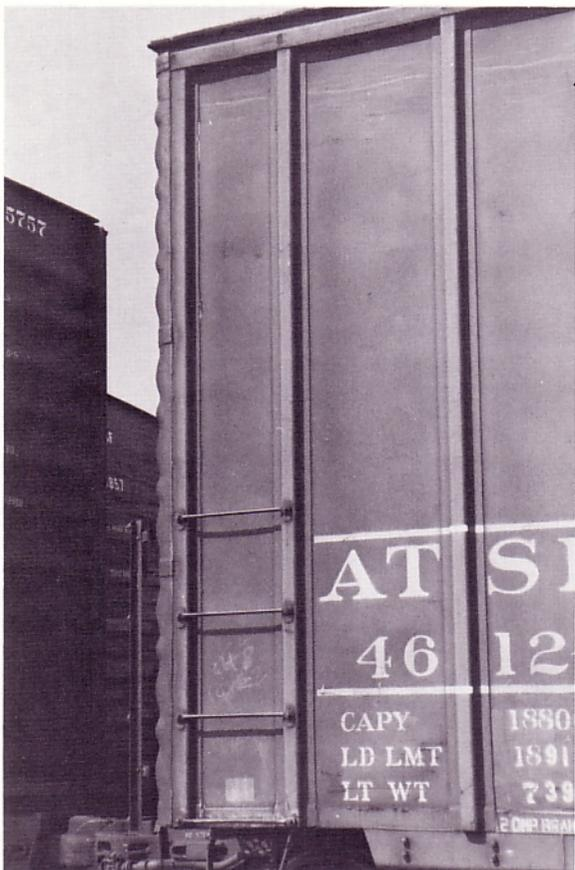
End-to-side joint of the **ACF 6100** design showing the welded wrap-around construction. Note the thinner posts and wide flanges on this design versus the other two.
