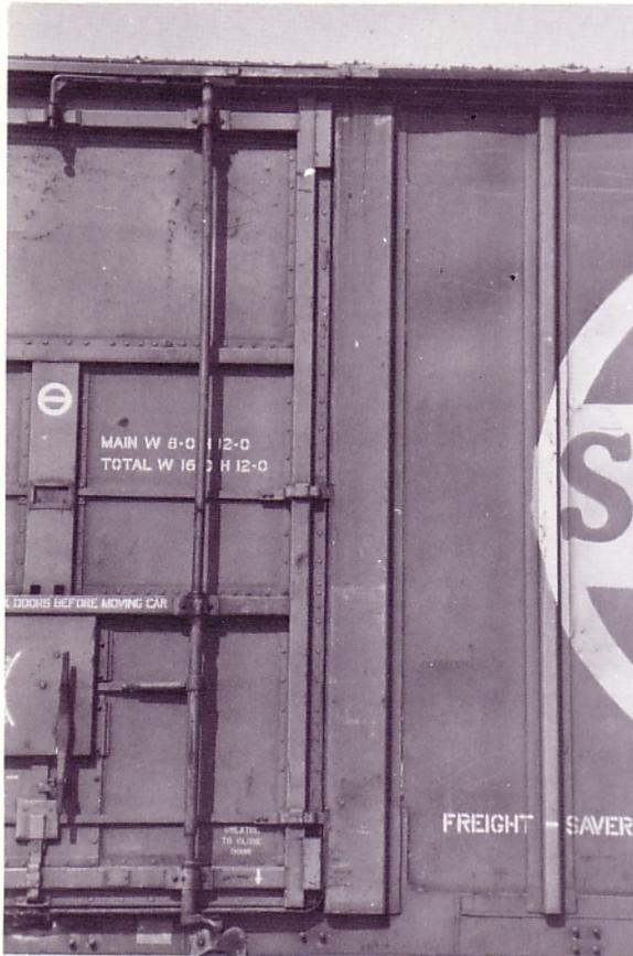
Door post of the PS 6196 design. Note how it's similar to the other posts on the sides and narrower than the Berwick style.
