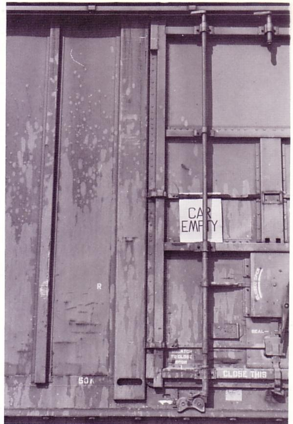
Door post (the post adjacent to the door) of the BFF 6196 design. Note the wider design and the oval opening at the bottom.
