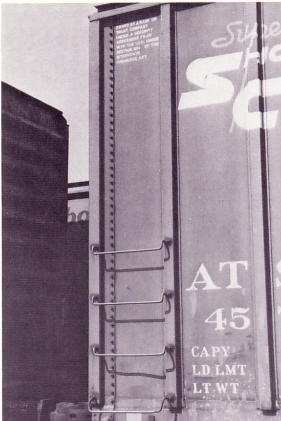
End-to-side joint of the **BFF 6196** design shows the riveted construction. Also note the shape of the posts.
