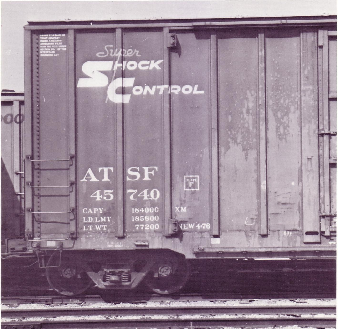
An additional view of the BFF 6196 design showing the 5 posts on one side of the door and the "X" style roof panels.
