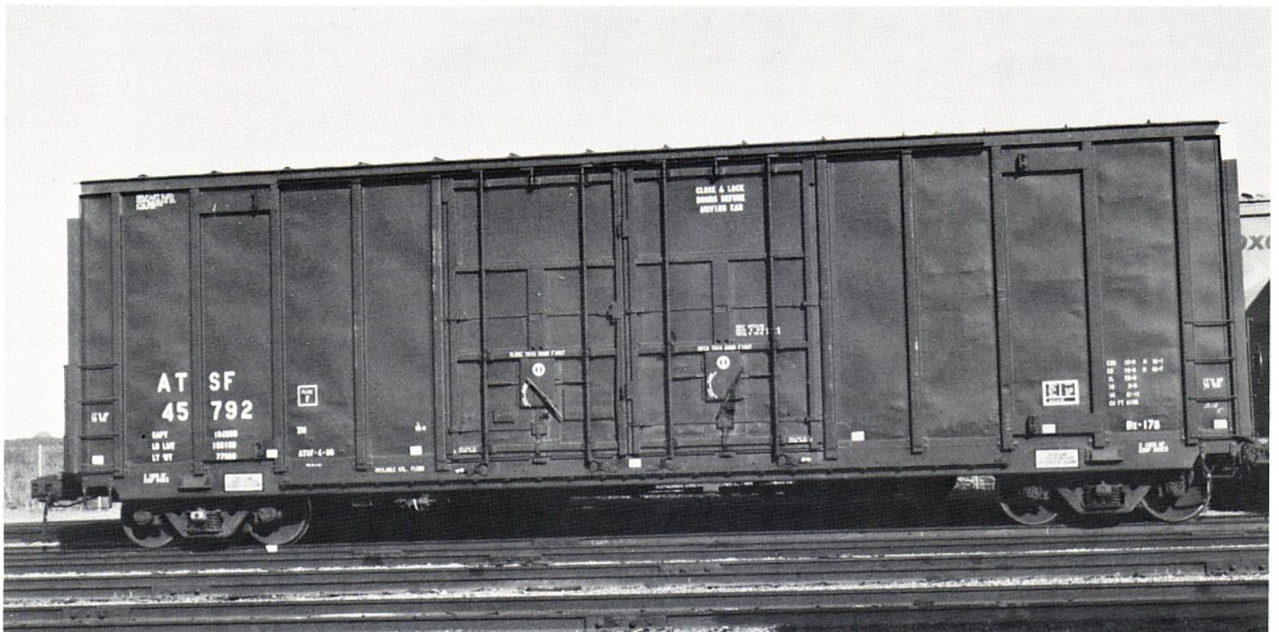
*PS 6196. ATSF 45792 as it appears in the latest livery. Note the 8-post (referred to in the table under sides) welded construction.*
