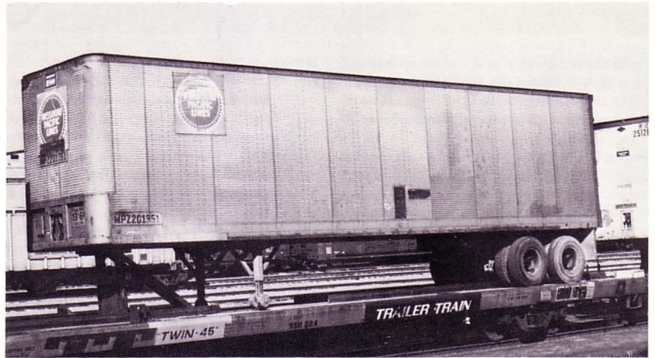
MPZ 250110. Trailmobile's 45-foot piggyback van. Note the use of two sets of reporting marks and numbers on the sides of the vans, an unusual practice for modern pig vans but common to later MP piggyback trailer liveries.
