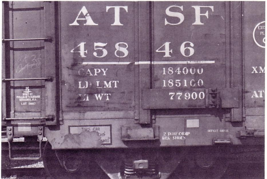
Side sill architecture of the **PS 6196** design. Note just the short line to almost the first post and then angled and dropped.
