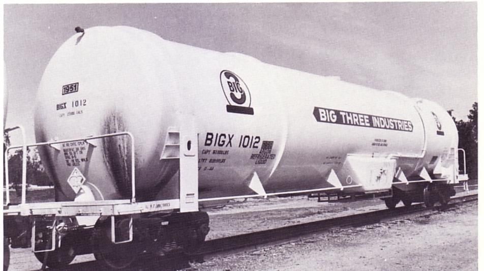
**BIGX 1012-1014.** Built in 11-80 by Process Engineering, Inc. in Plaistow, NH (abbrev: PEI NH). This series has a 25,840 gallon per car capacity.
