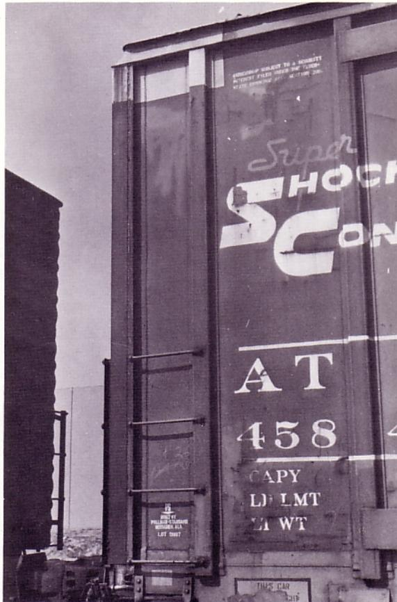
End-to-side joint of the **PS 6196** design showing the welded construction. Note the design of these posts compared to the Berwick design (more similar) and the ACF design (less similar).
