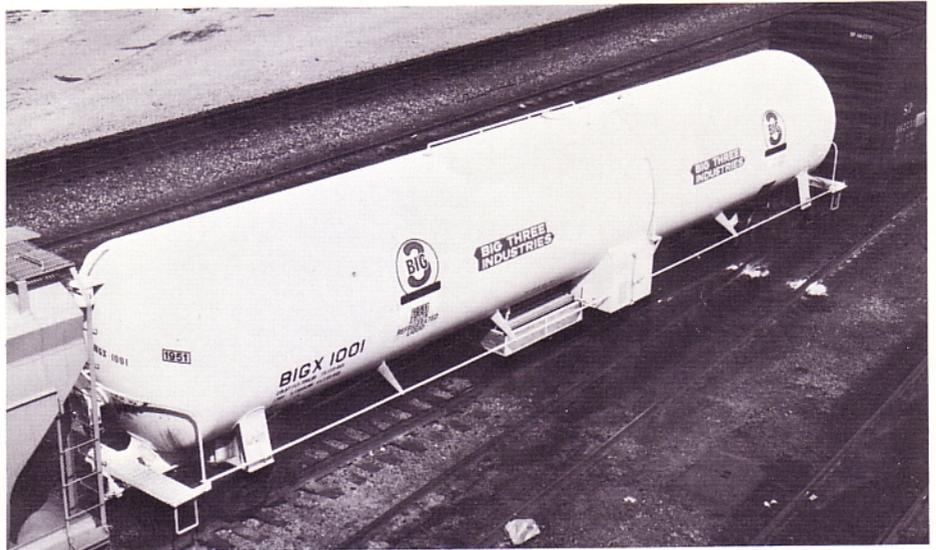
*(RIGHT) BIGX 1001. Built in 1-69 has a 25,471 gallon capacity. All of the BIGX cars are used for refrigerated liquid argon. This top view shows the lack of typical tank car inlets. Only a small manway is barely visible near the center of the car on top.*
