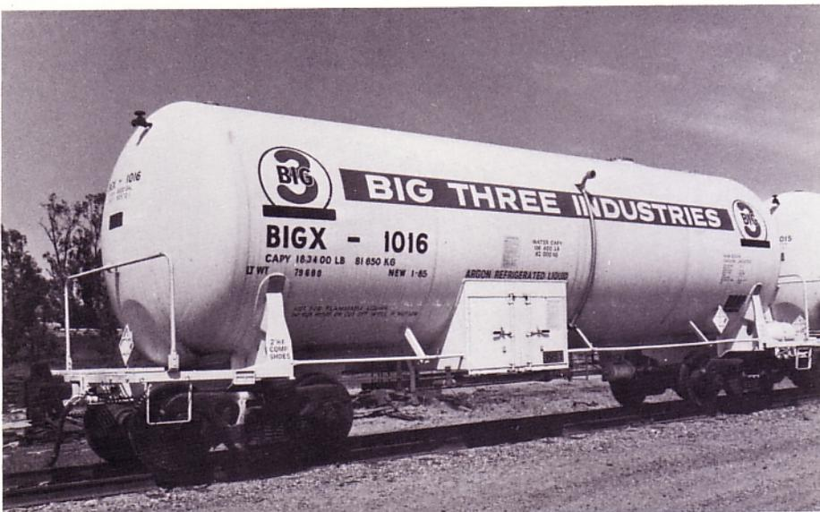
***BIGX 1015-1016.** The frames were built in 9-84 by American Car & Foundry's Milton, PA plant. The tanks were built and assembled to the cars in 1-85 by Process Engineering Inc. These cars have a 16,530 gallon capacity.*
