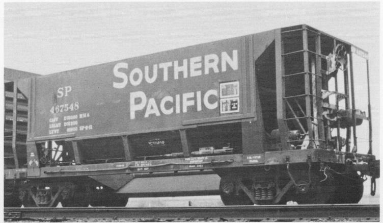
SP 467548 is a Thrall Car built hopper, one from the only series of ore cars in the fleet. Pat A. Holden
