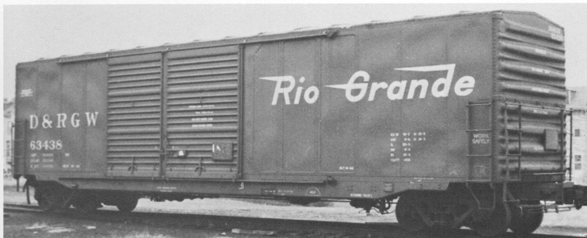
DRGW 63438, an ACF built double door box car with wood lining and nailable steel floor. Seen in this view at Reading, PA on November 17, 1968.
