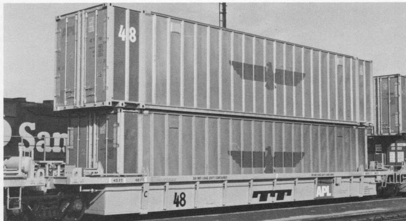
Left. DTTX 62403c, a Thrall built articulated double stack container car. Livery is TT yellow, black data and blue and white APL panel. Note the absence of "bulkheads" and ribbed sides for identification of this design. Notice the ribbed 48-foot container on top (the rarer of the three styles of 48'ers in production).
