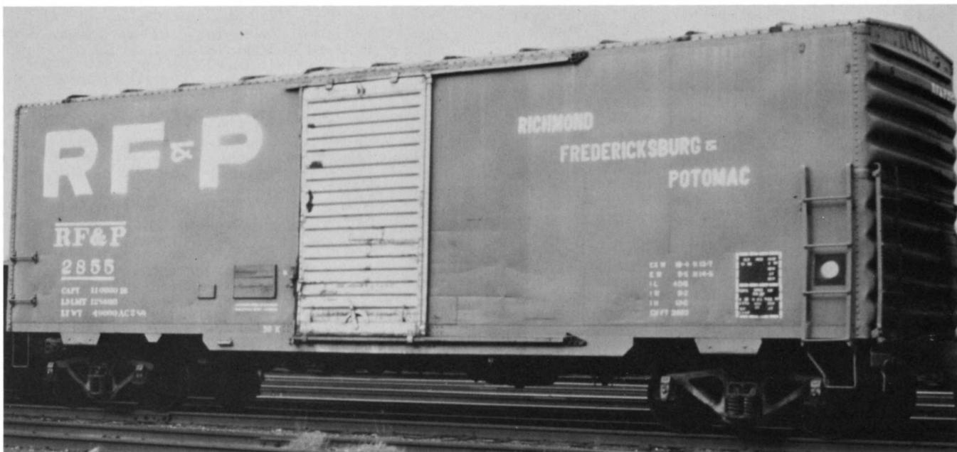
(Above) RF&P 2855, shown at Richmond 4-27-81. Built in 1952 by Pullman-Standard represents one of the few 40-foot boxcars operating with U.S. railroads in the 1980's. (Below) RF&P 8121, built in 1958 was acquired used by the RF&P. Shown here at Richmond 4-26-81. Both photos by J.R. Quinn
