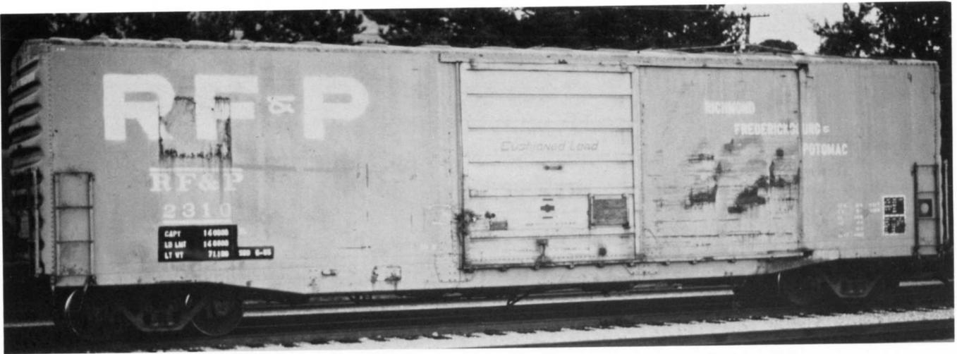
(Above) RF&P 2310 shown here in San Luis Obispo on 4-5-86 was built by Pullman-Standard in 1963. The car was scaled on the Seaboard System in 6-85. Door is aluminum, white lettering, data, logo. Light weight and capacity area was painted black after being scaled. Pat Holden photo
