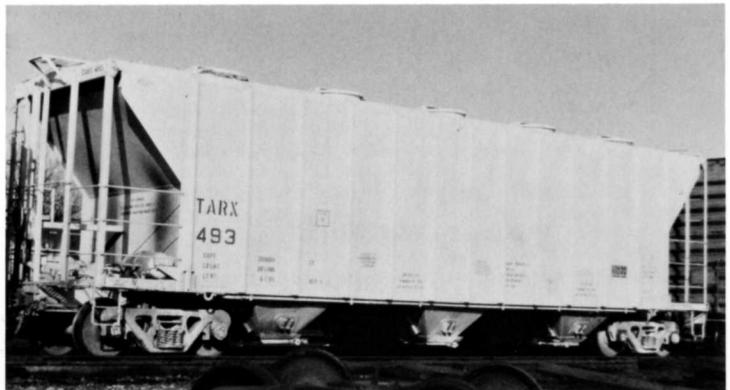
TARX 493, former SAN 493. TARX is the reporting marks for Sandersville Leasing, a subsidiary of the SAN. The cars were rebuilt in 1981 by the Safety Railway Service. Note the lack of the large Sandersville logo and large number used on SAN initialed cars. This car has the centered roofwalk. covered hoppers later received by the Sandersville had off-centered walks. Tony Hodun photo
