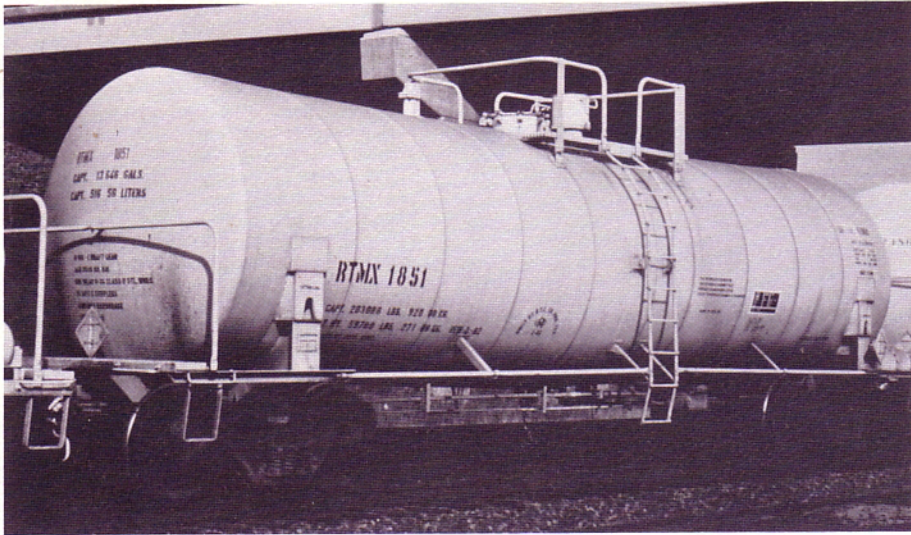
RTMX 1851, 100-ton tank car with 13,646 gallon capacity. Built by Richmond Tank Car, Houston, TX and leased by Richmond Leasing to OMYA, Inc. for limestone slurry transportation. Light weight 59700. Built 2-82. White tank with black lettering and data. Tony Hodun photo
