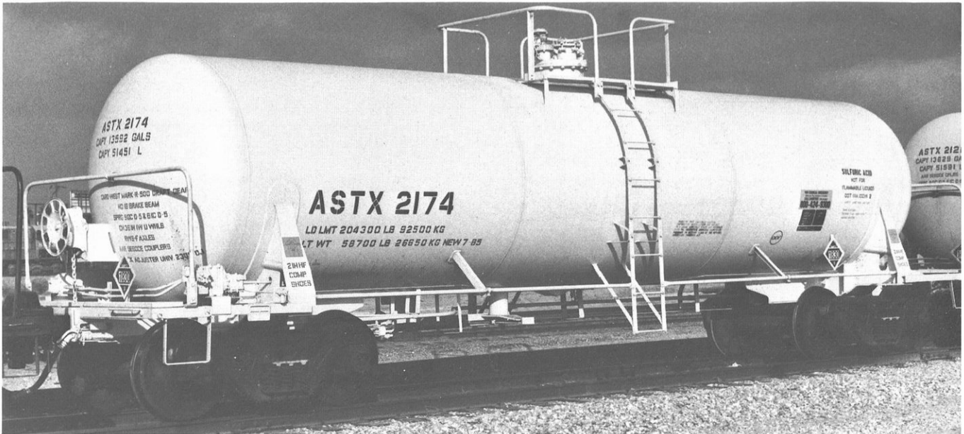
Asarco's ASTX 2174 an ACF built sulphuric acid tank car. Livery is white with black lettering. David G. Casdorff photo
