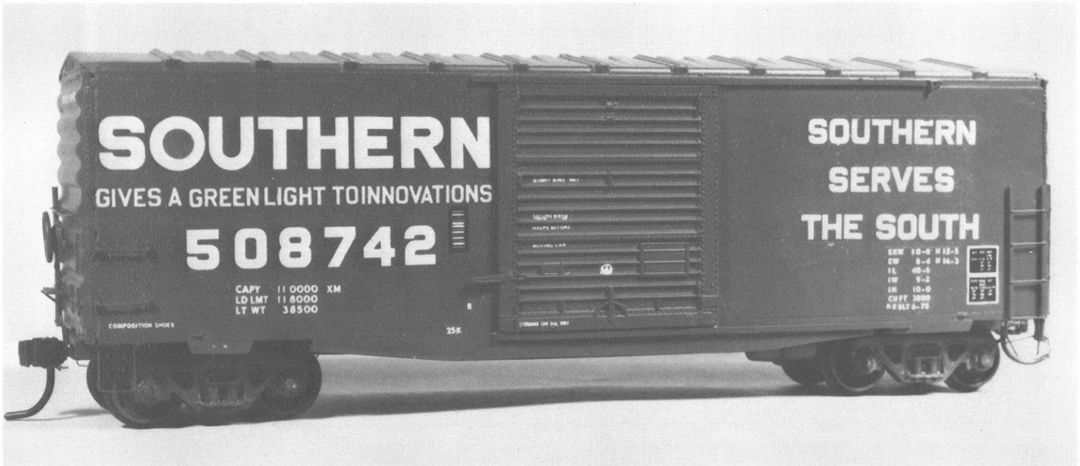
Model car no. 508742 is built up over an Athearn grainloading box car body with diagonal roof panels, side overlays scribed to represent welded construction, narrowed Athearn doors and CCS Pullman type ends (Staffan Ehnbohm photo)
