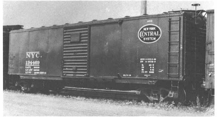
NYC 134469, Lot 695B. This is a 1916 all-steel box car as rebuilt in 1941 with a single door and new roof.
