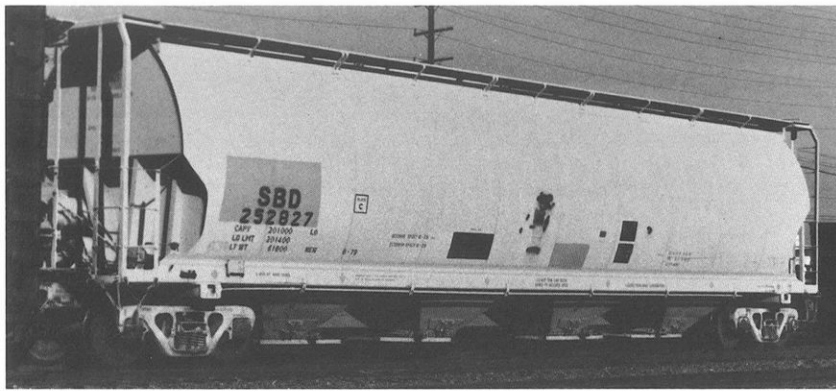
Seaboard 252827, a National Steel Car built 100-ton covered hopper recently acquired from the Warrenton RR. David G. Casdorff photo
