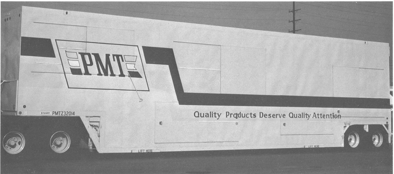
PMTZ 32014, a new "piggyback" trailer for transporting automobiles. Built by Stuart (builders of truck auto carriers). Shown at Industry, CA in January 1986. Ed Flaughner photo
