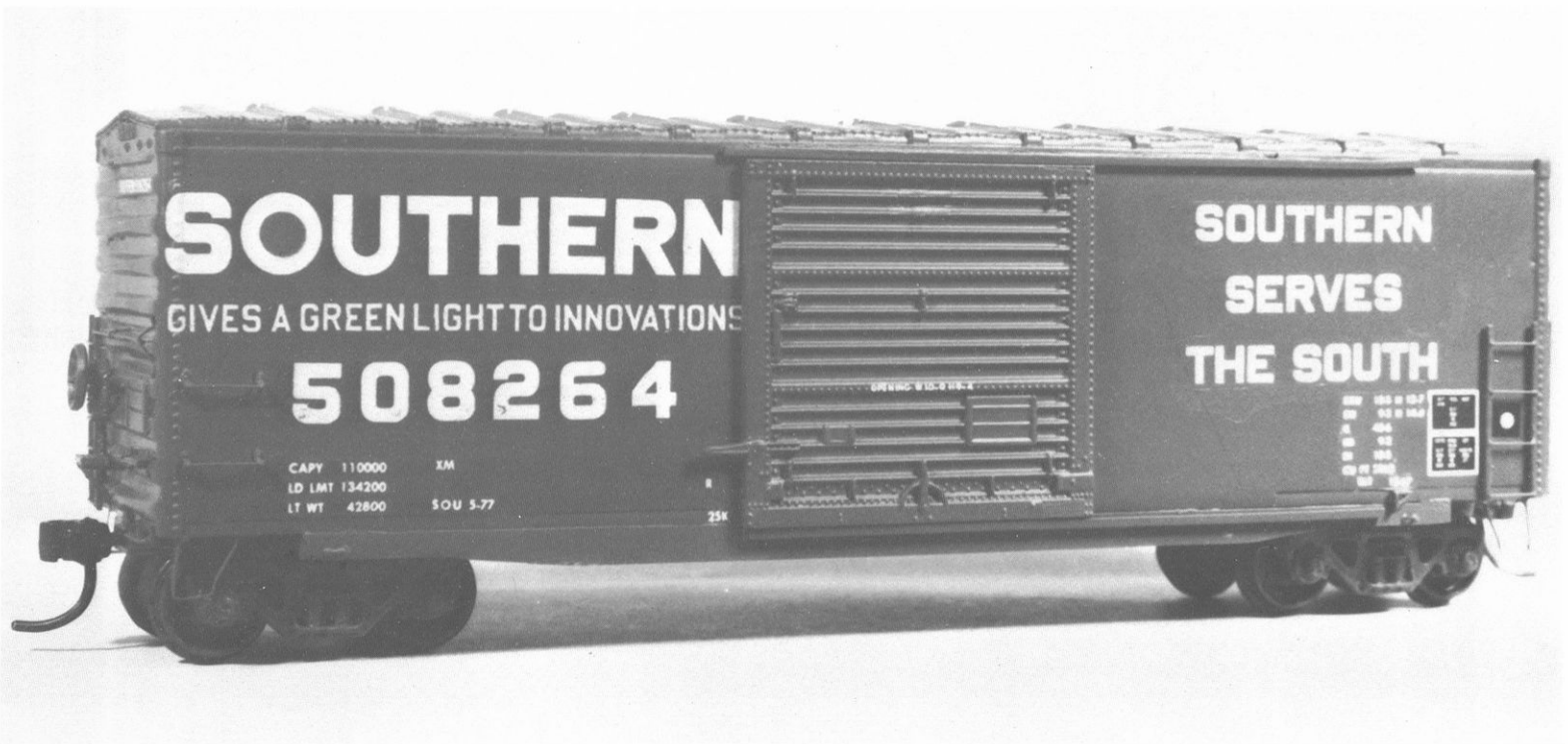
Model car no. 508264 is an AHM car with an Athearn Railbox door and a new side sill and details (Staffan Ehnбом photo)
