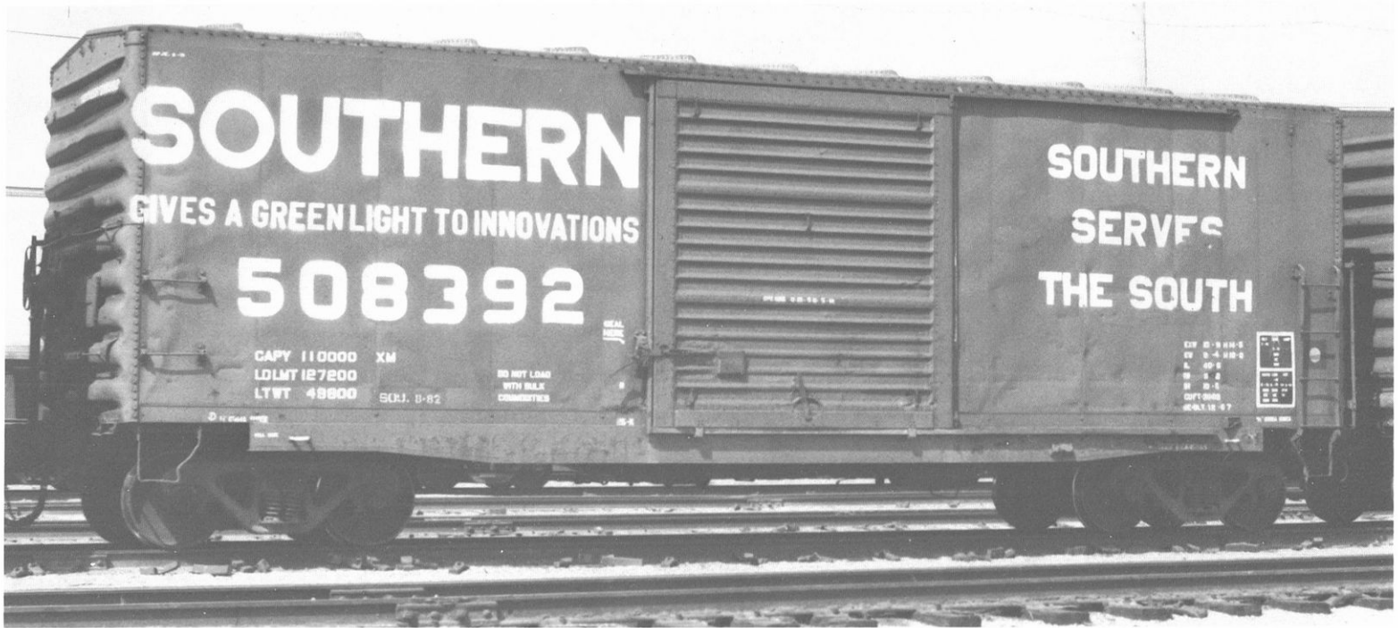
Prototype car no. 508392 is the prototype for the easy model. The car has typical Pullman details including the roof panels. The door seems to be a later addition. (Red Davis photo)
